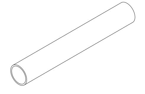
Perpendicularity call out on end of tube is so we'll have a square edge when we use this edge as a trim guide. Face this if the stock tube wasn't cut square enough.
