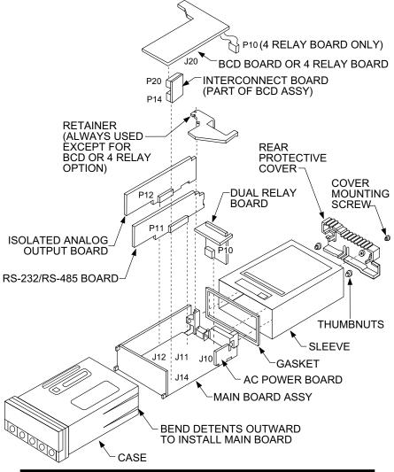
Figure 5-4. Optional Printed Circuit Board Locations
