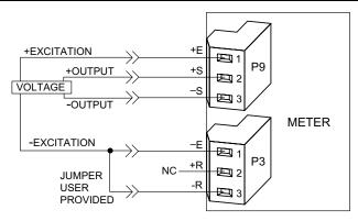
Figure 7-5 4-Wire Voltage Input With Sensor Excitation
