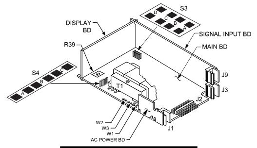
Figure 5-6. ac-Powered Main Board
