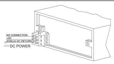
Figure 7-9. DC Connector Wiring at P1
