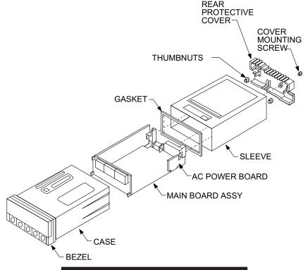
Figure 5-1. Meter Exploded View
