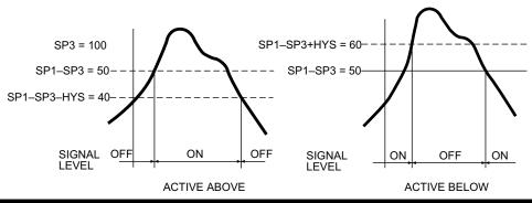
Figure 10-5. Low Deviation for both Active Above and Active Below
