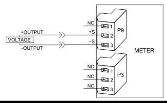
Figure 7-3. Voltage Input Without Sensor Excitation
