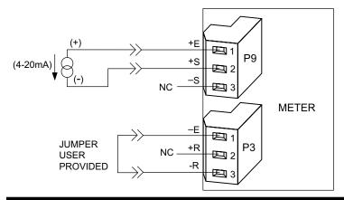
Figure 7-2. Current Input With Sensor Excitation
