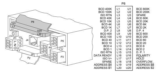
Figure 13-1. BCD 40-Pin Cable Connector (P8)
