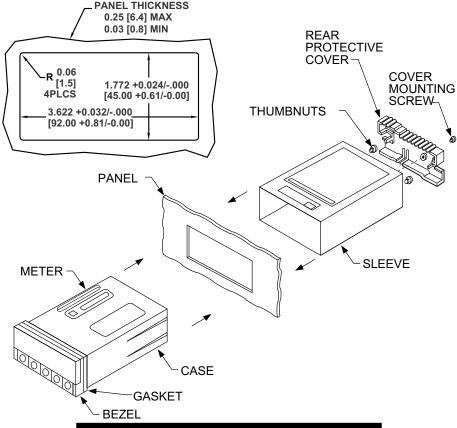
Figure 5-14. Panel Mounting Assembly
