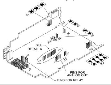
Figure 6-3. dc-Powered Main Board Jumper Positions S3 and S4
