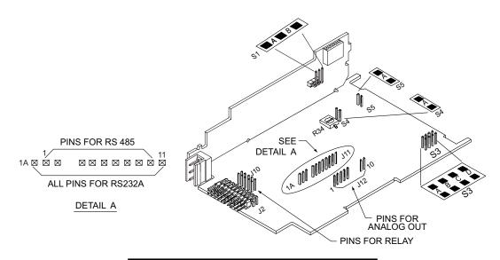
Figure 5-7. dc-Powered Main Board
