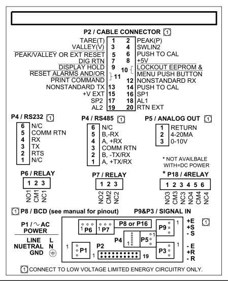
Figure 4-2A. AC Power - Connector Label for Rear Connectors
