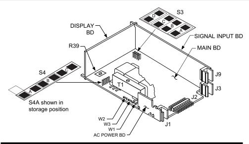
Figure 6-2. ac-Powered Main Board Jumper Positions S3 and S4
