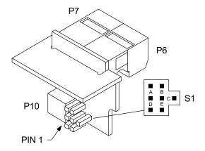
Figure 5-8. Relay Option Board
