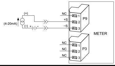
Figure 7-1. Current Input Without Sensor Excitation
