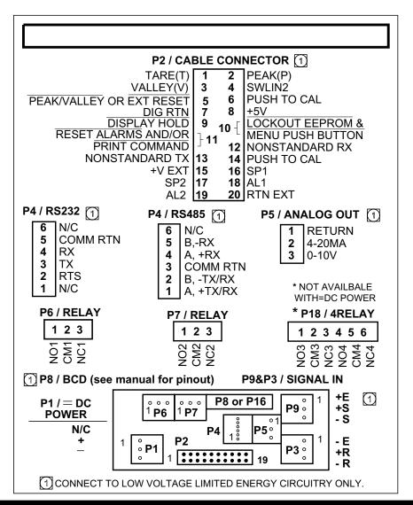
Figure 4-2B. DC Power - Connector Label for Rear Connectors
