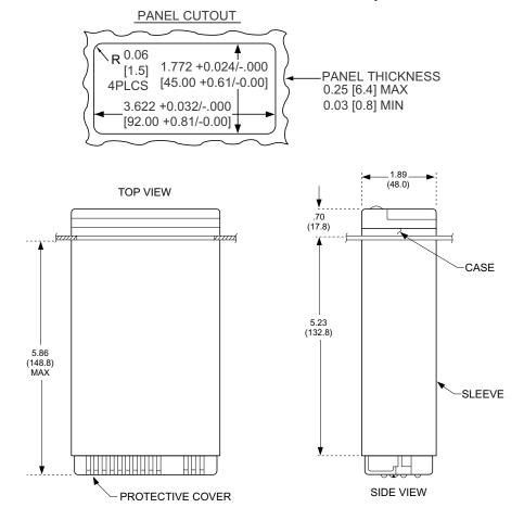
Figure 18-1. Meter Housing and Panel Cutout.
