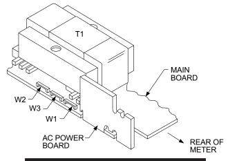
**Figure 5-3. Transformer Jumpers**
