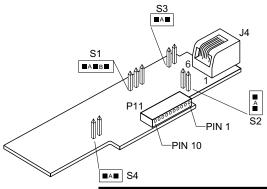
The RS-485 option board has been updated. The figure shown is an older version, the newer version is the same figure as the RS-232 option card shown above.
