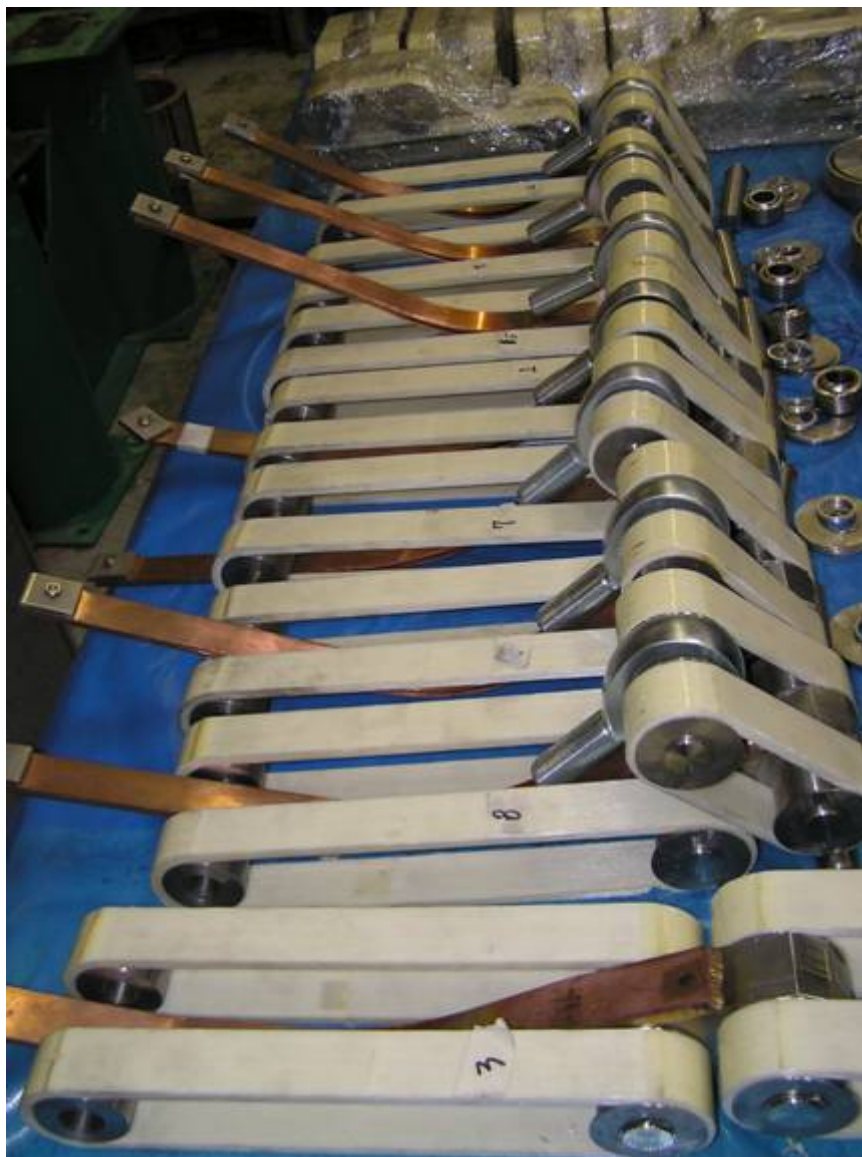
Cold mass supports with four fiberglass links and copper strap for shield intercept
