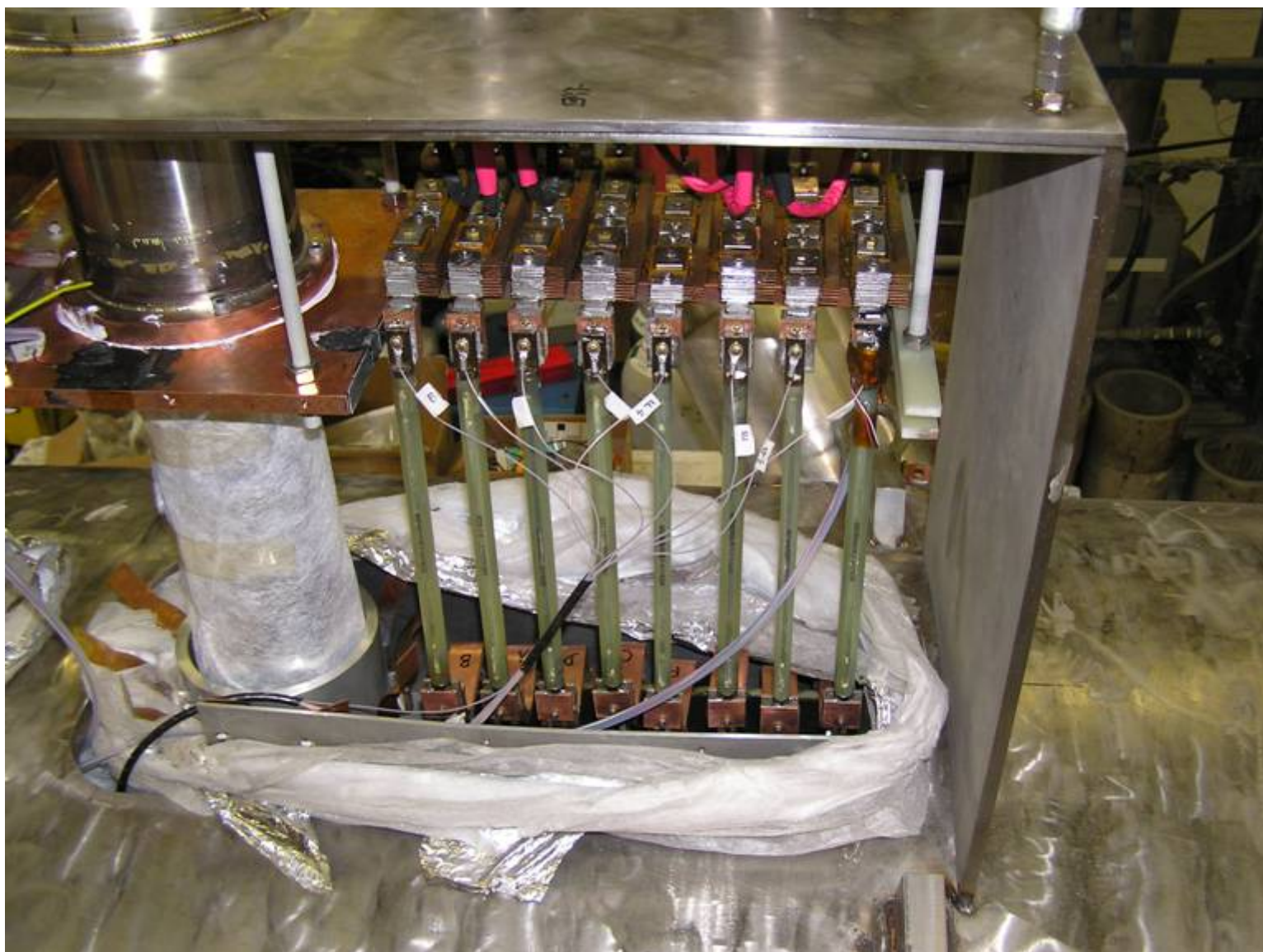
Upper leads and HTS leads assembly in magnet turret
