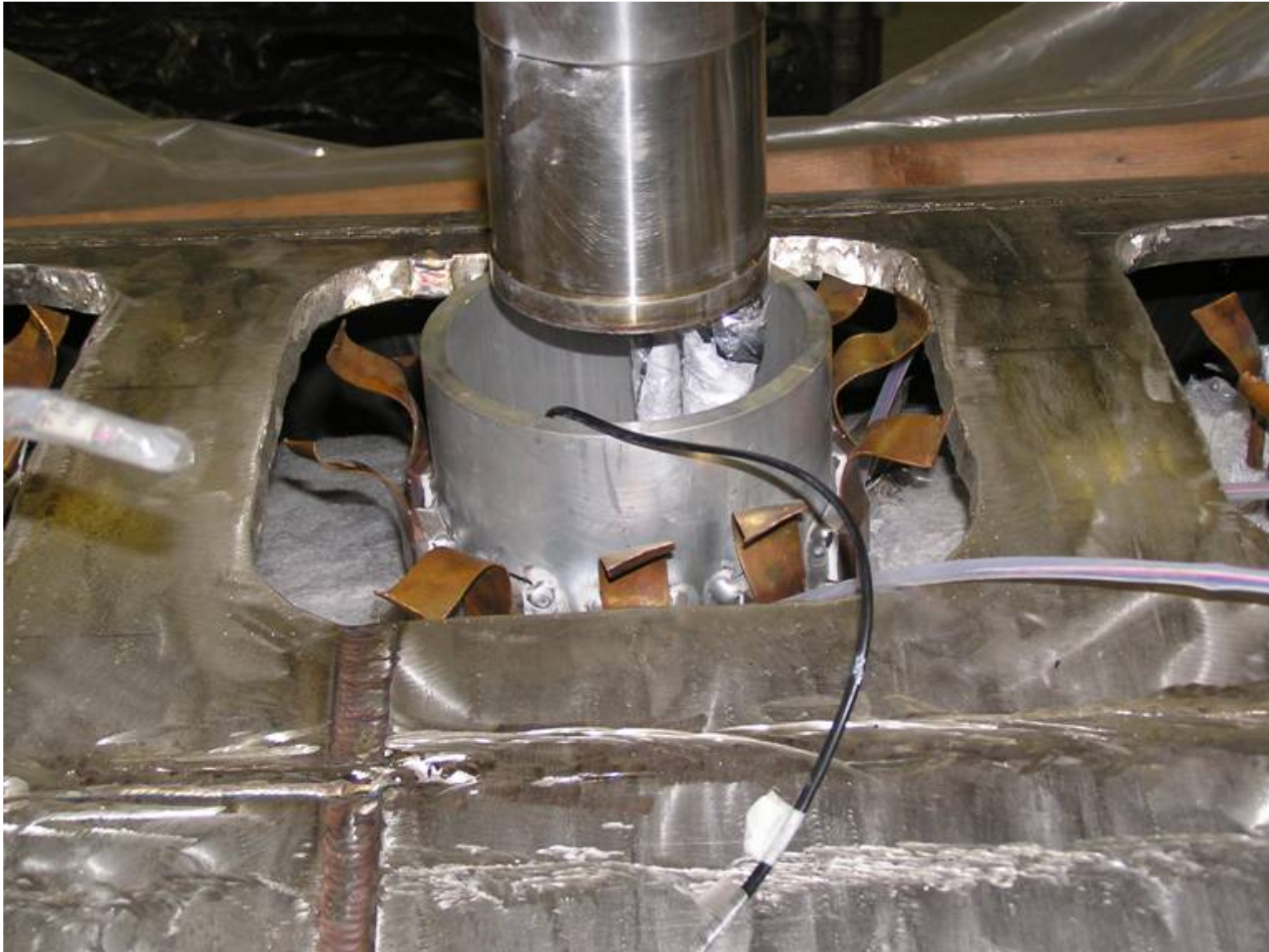
Cryocooler 1 st stage sleeve attachment area (Magnet 1 w/thin Cu instead of thick 1100 Al)
