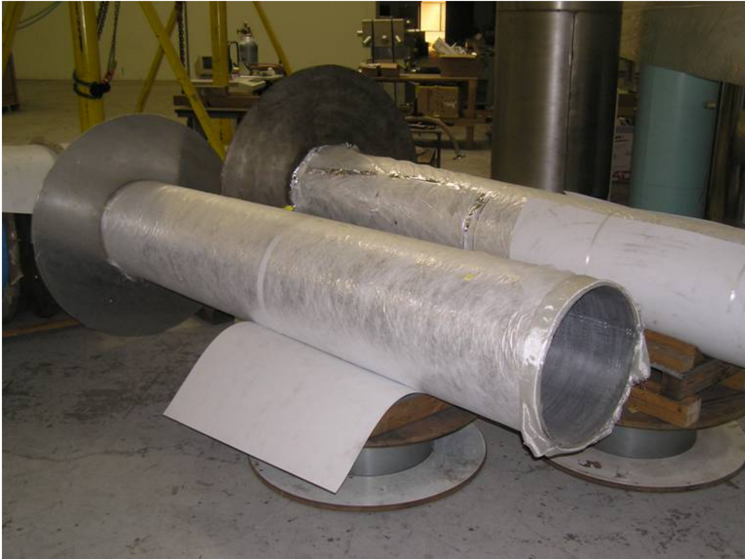
MLI wrapping on OD of thermal shield inner bore (left) and on OD of vacuum vessel inner (warm) bore (right)
