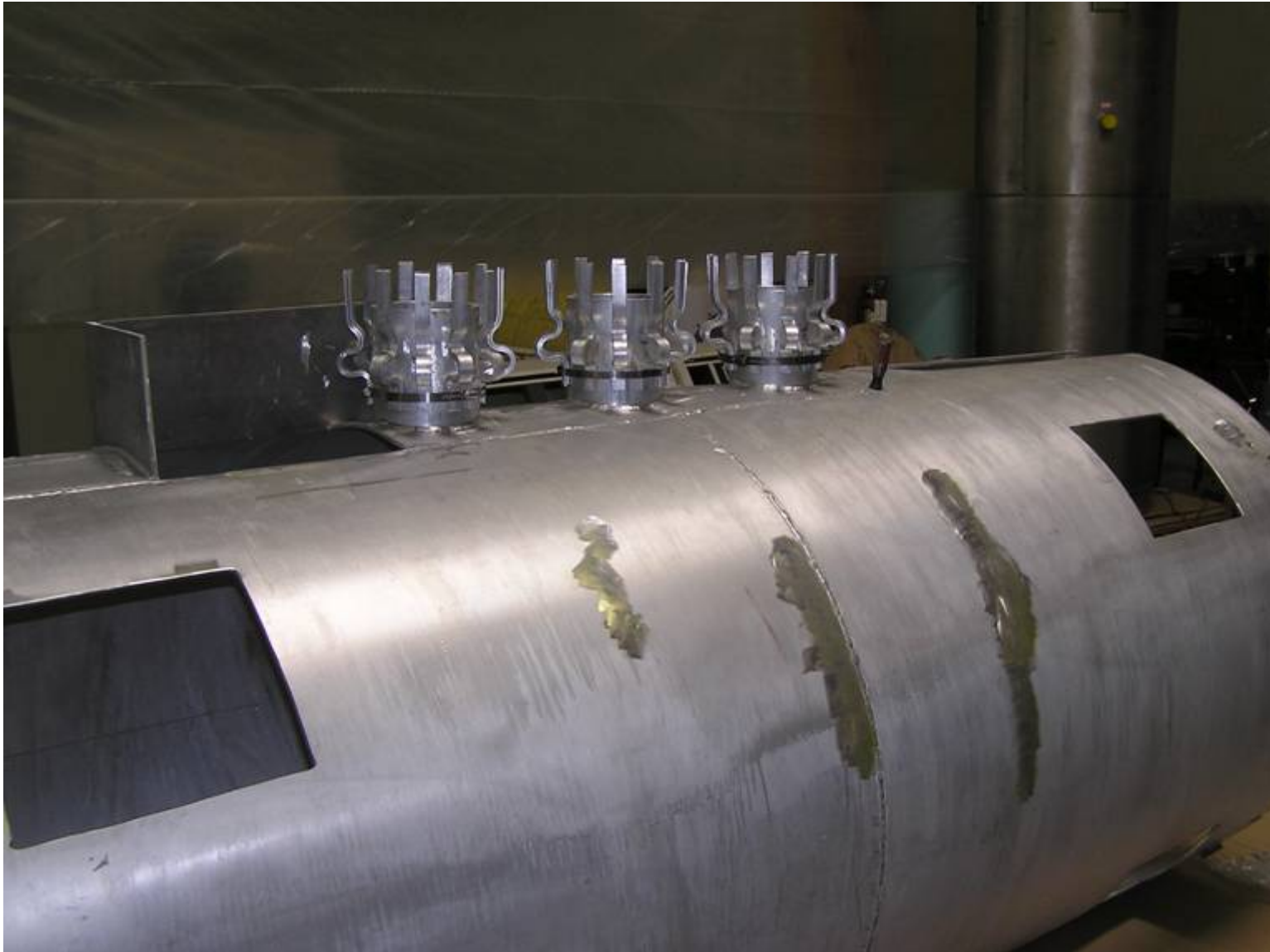
Magnet thermal shield showing connections to cryocooler cooler 1 st stage sleeves
