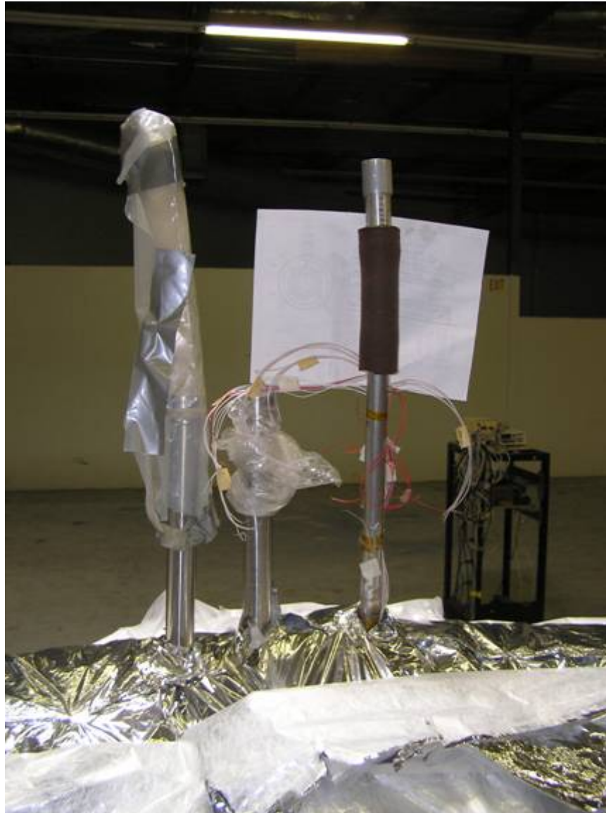
Cold mass fill and vent lines (w/instrumentation wires) for Magnet 1 (2 nd iteration)
