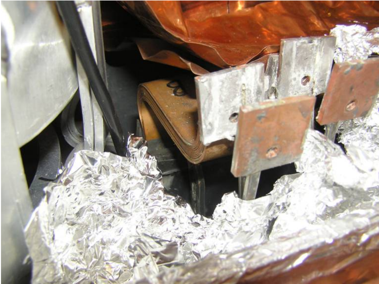
Close up showing coil tap and thermal intercept for lower end of HTS lead
