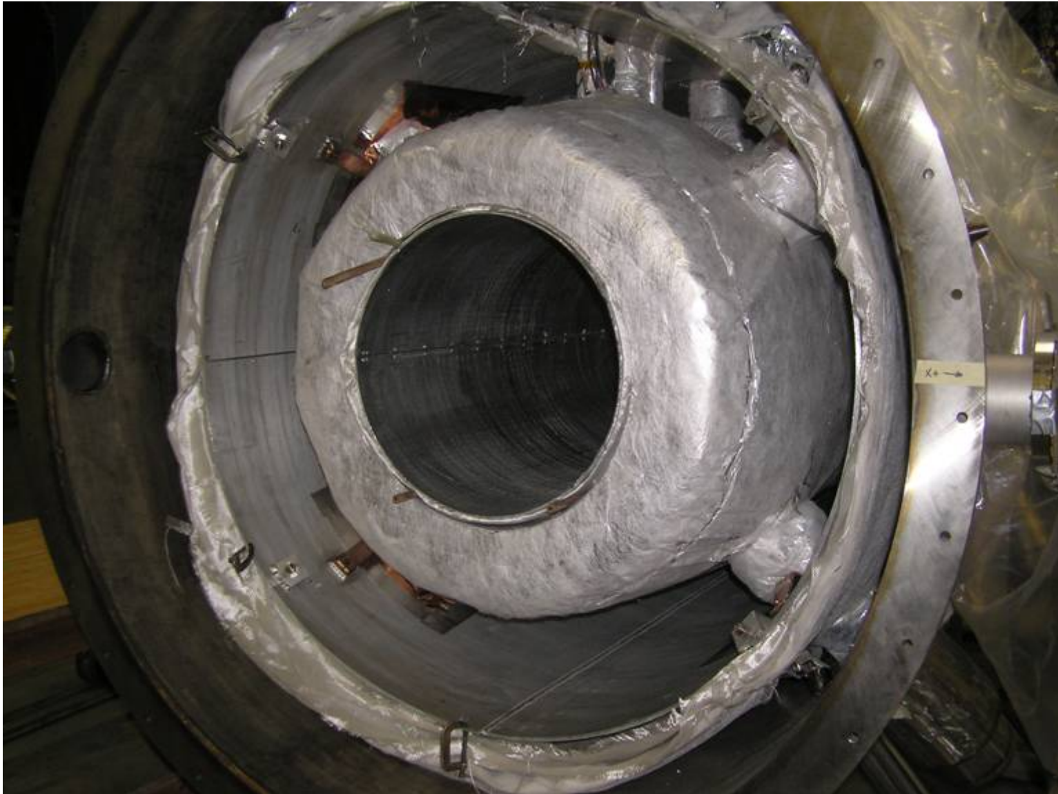
Close up of cold mass ends showing wrapped cold mass supports
