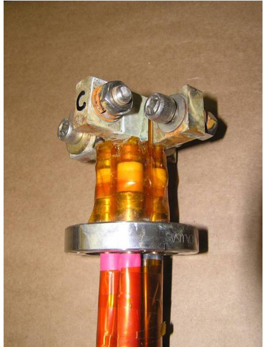
Upper leads and feedthrough for connection between 300K and 70K
