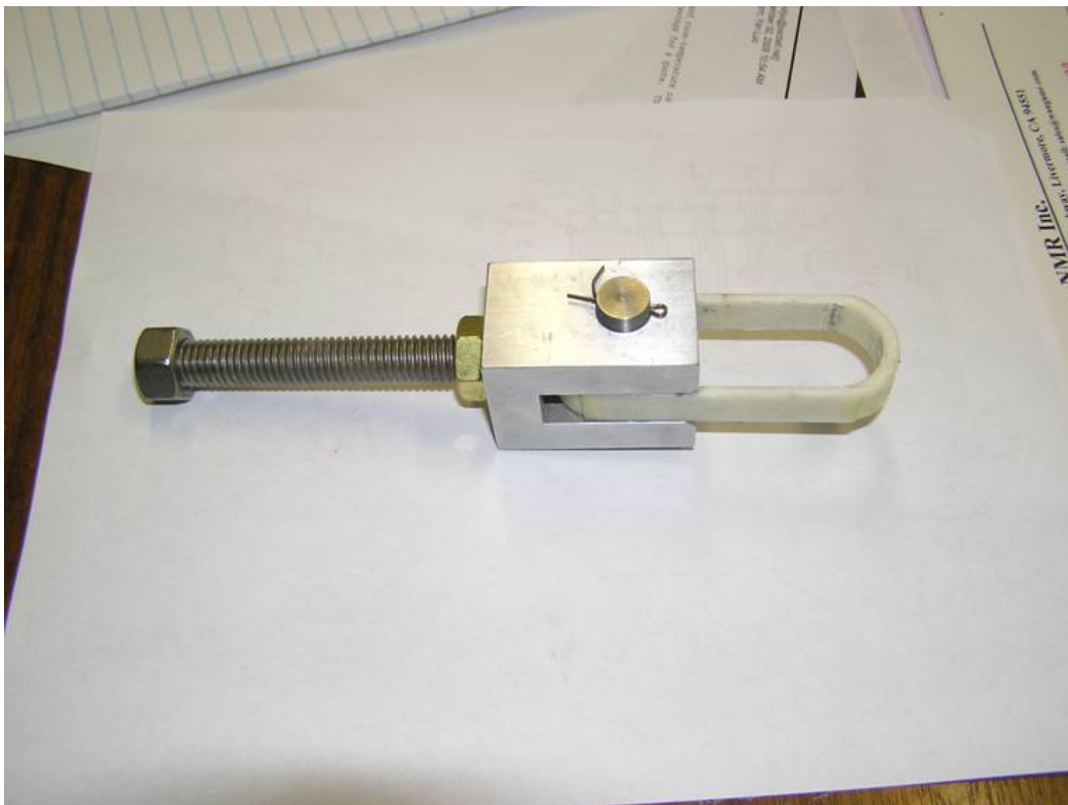
Fiberglass support band and clevis for thermal shield (4 at each end of shield)
