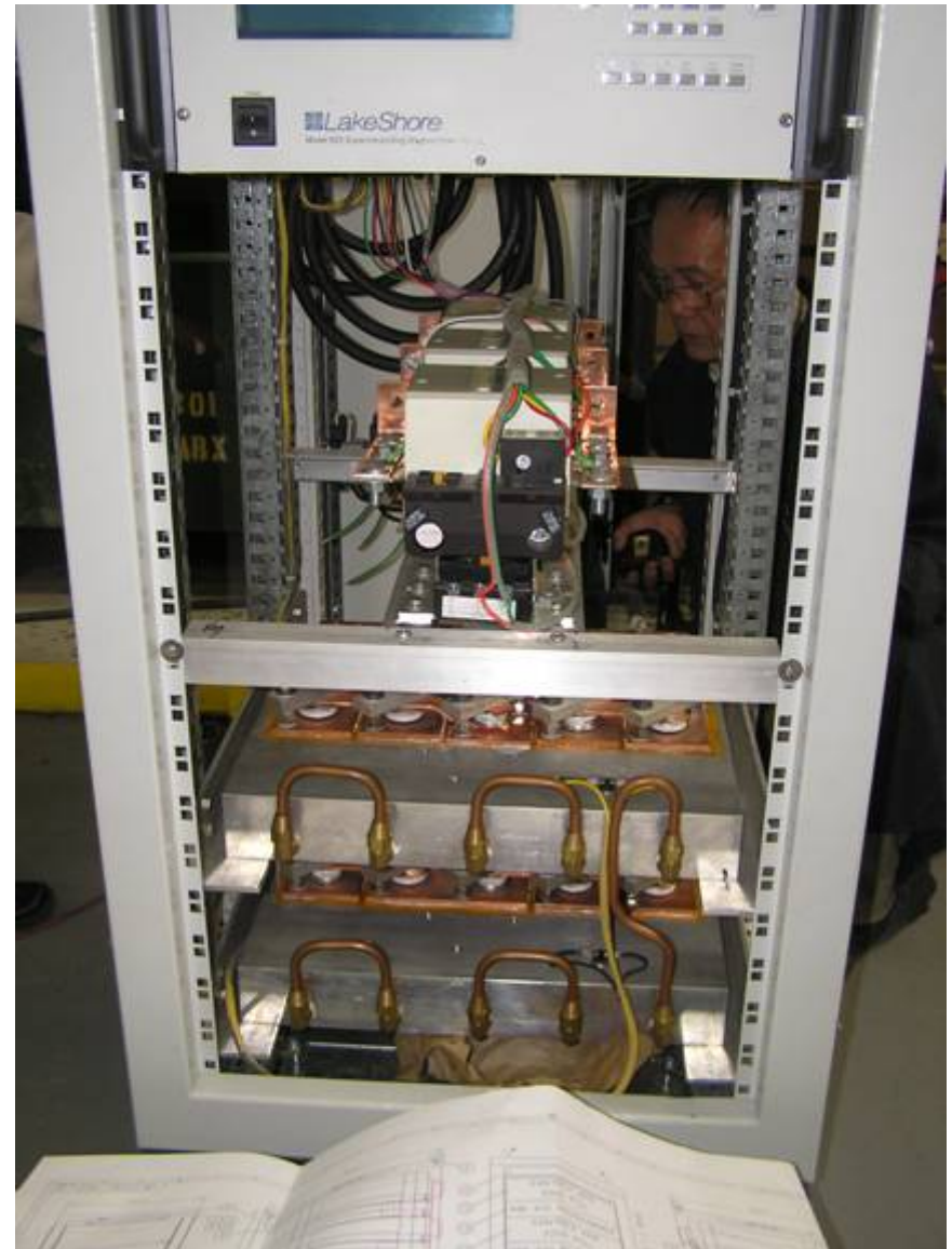
Front and side views of switches and power absorbing blocks for magnet discharge circuits
