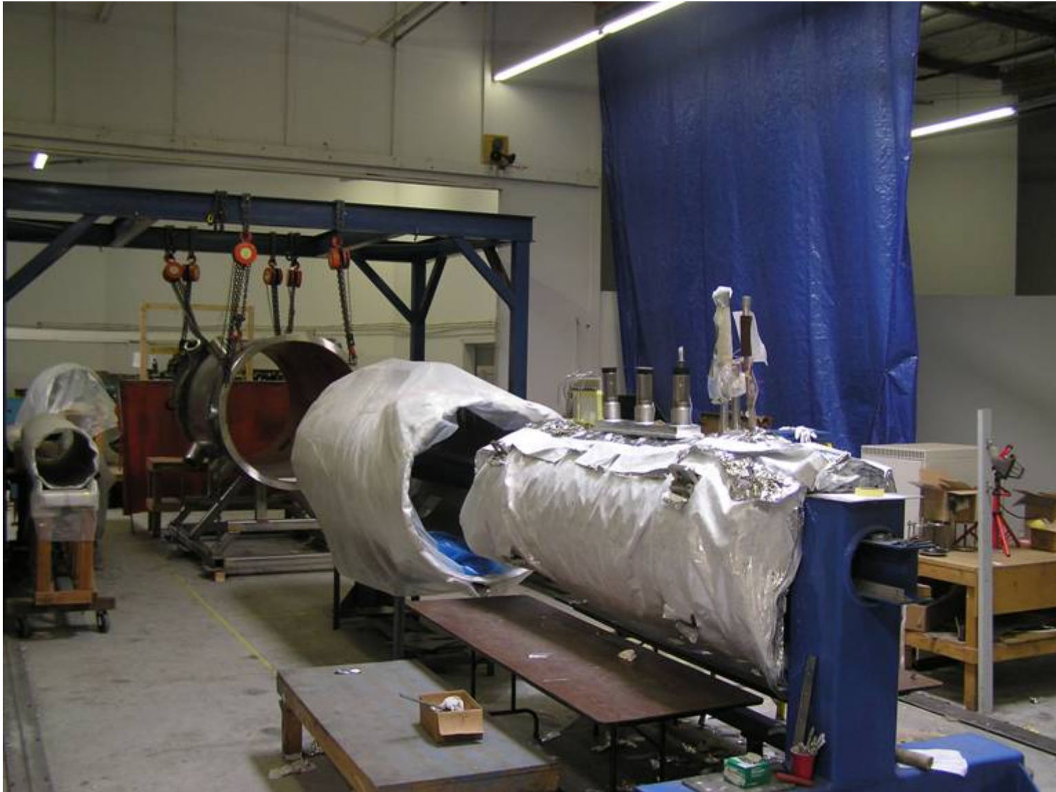
Preparation for assembly of Magnet 2 cold mass into thermal shield and vacuum vessel
