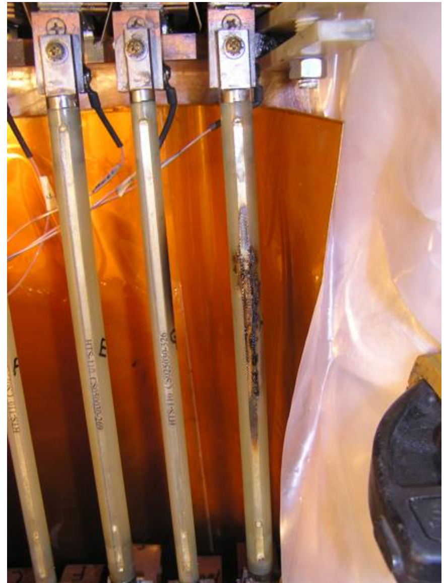
Magnet 2 HTS leads array showing burned out lead at far right
