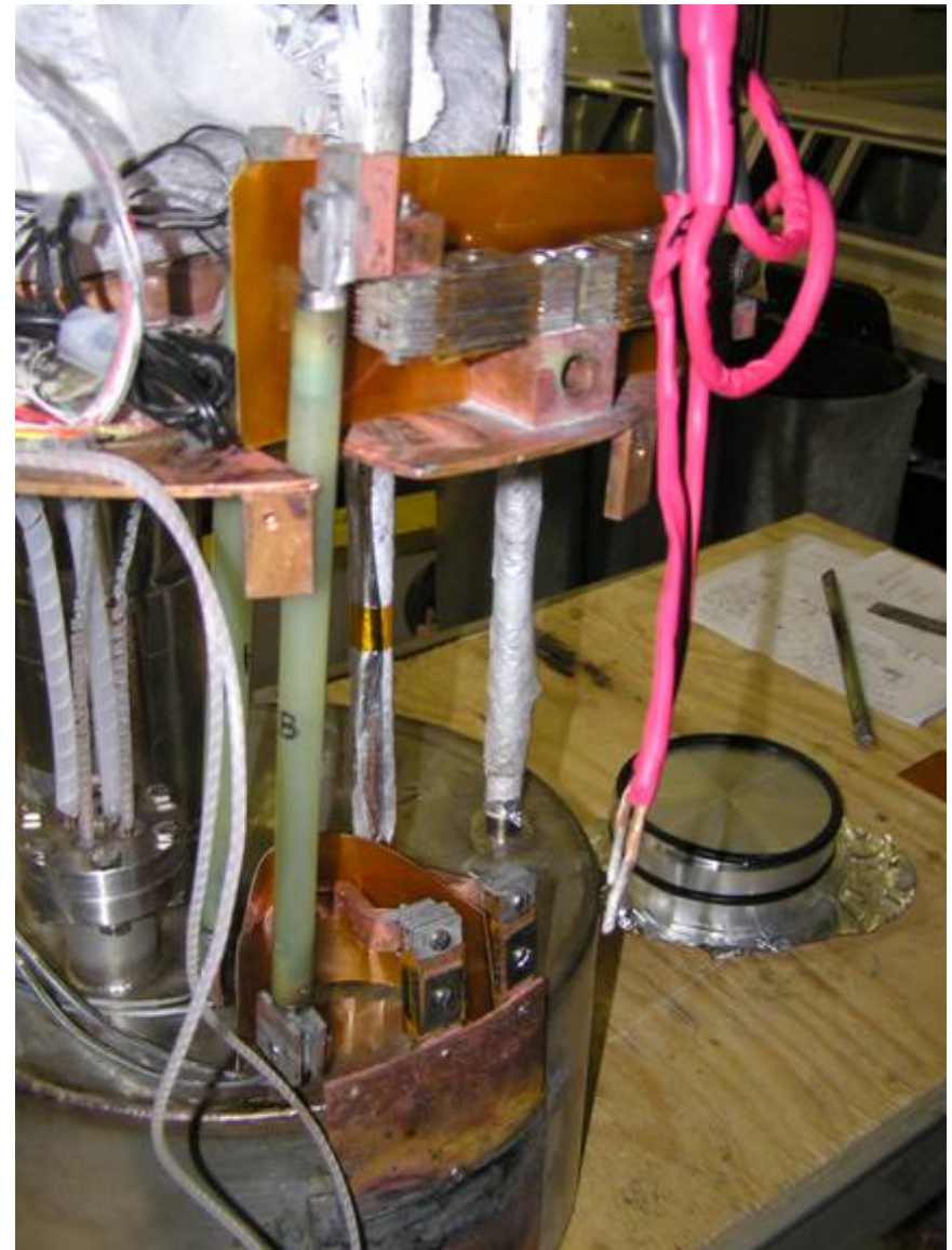
Cryocooler test rig modified to measure lead voltages and temperatures during operation
