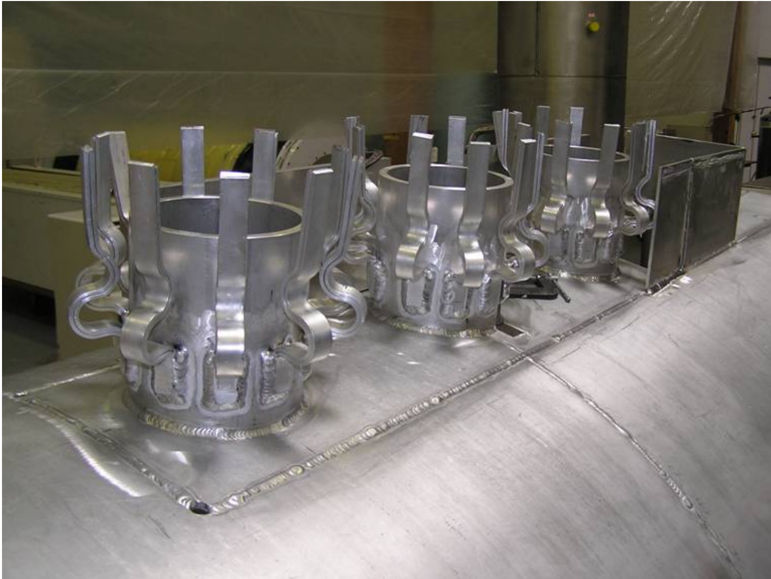
Close up of connections to cryocooler cooler 1 st stage sleeves (sleeves not in place)
