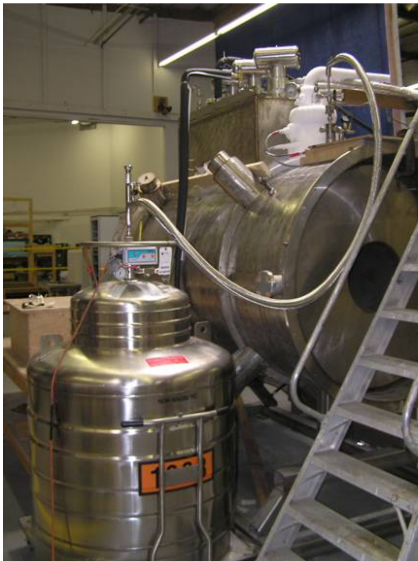
Magnet cooldown using liquid helium (Magnet 2)
