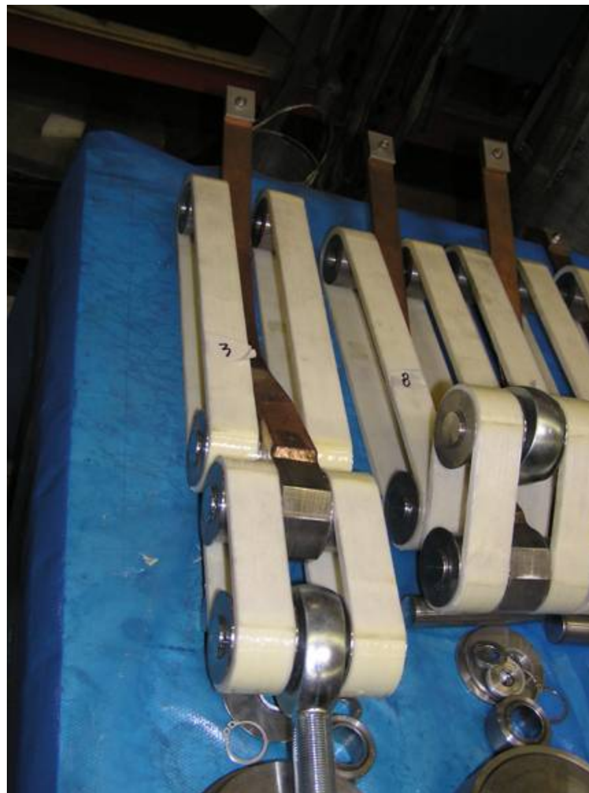
Cold mass supports with four fiberglass links and copper strap for shield intercept
