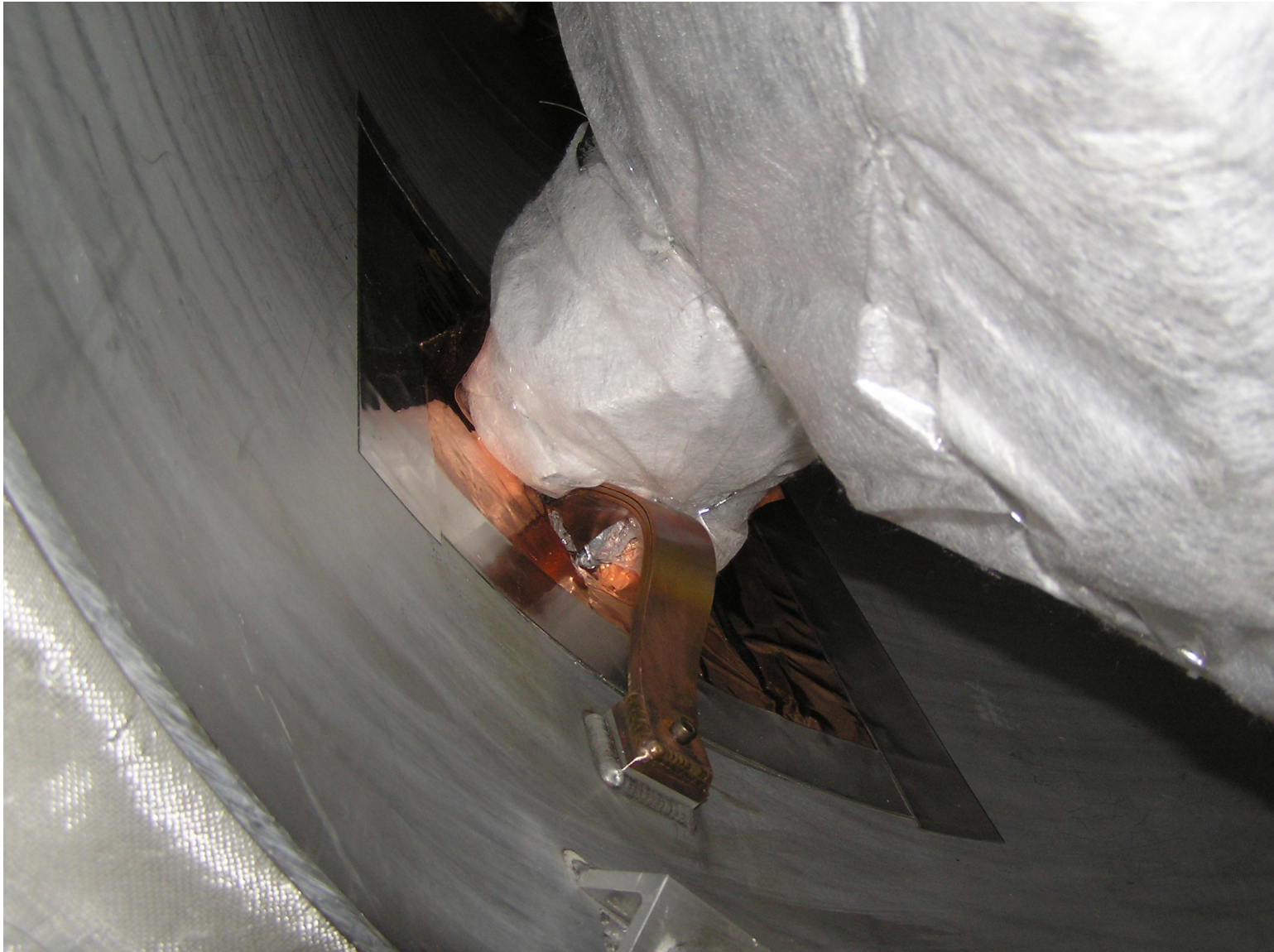
Cold mass support copper strap connection to thermal shield
