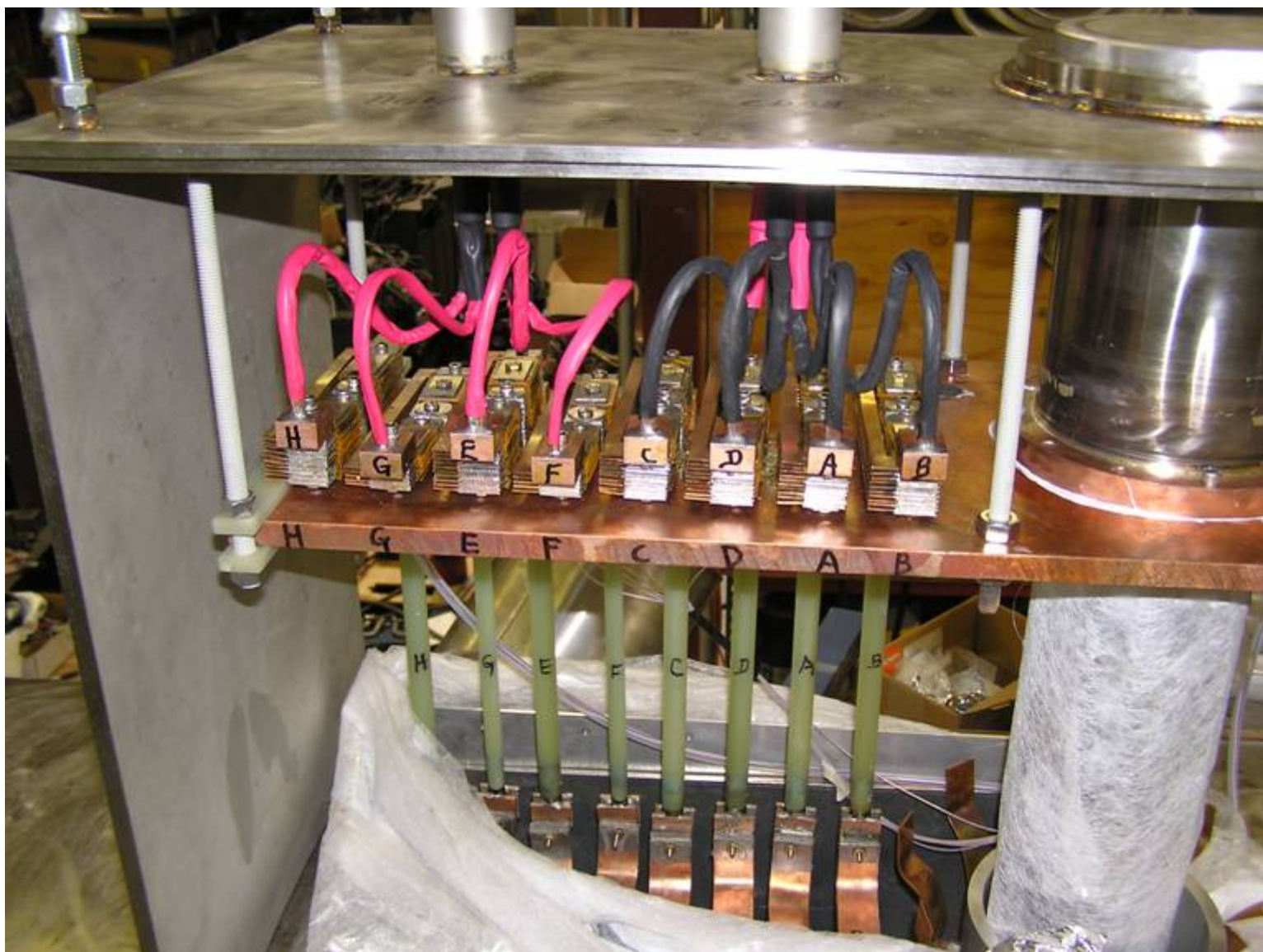
Upper leads detail showing thermal intercepts at 1 st stage cryocooler plate
