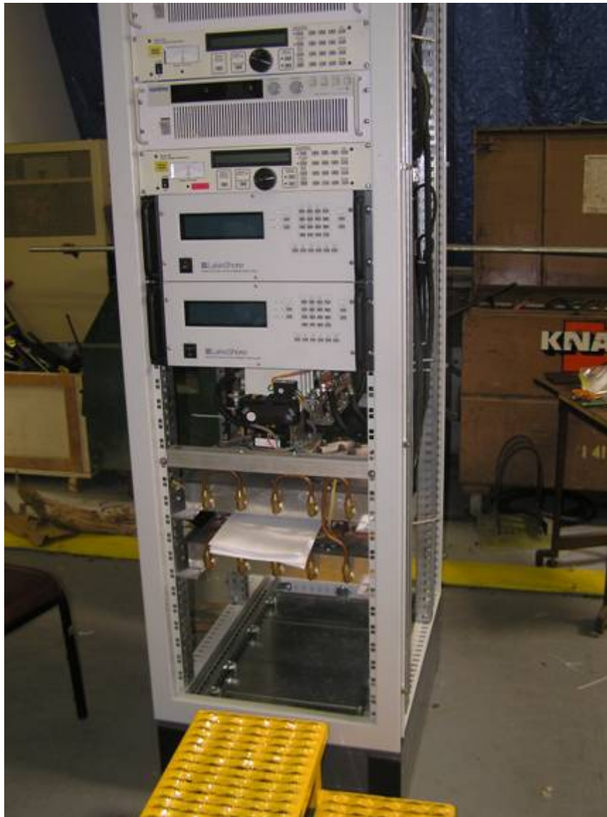
Front and rear views of assembled RAL racks for powering a single Spectrometer Solenoid
