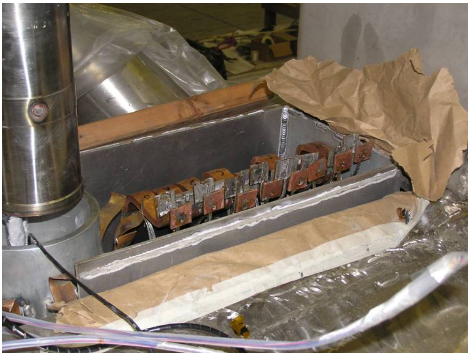
Coil taps and thermal intercepts for connection to lower ends of HTS leads
