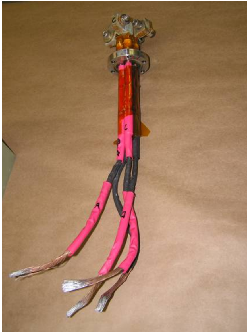
Upper leads and feedthrough for connection between 300K and 70K
