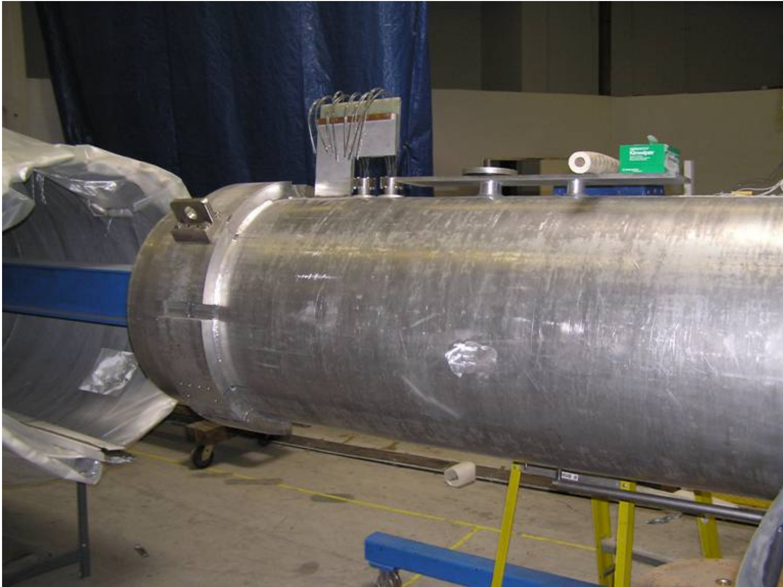
Final assembly of cold mass feedthroughs (leads and cooler ports, Magnet 2)
