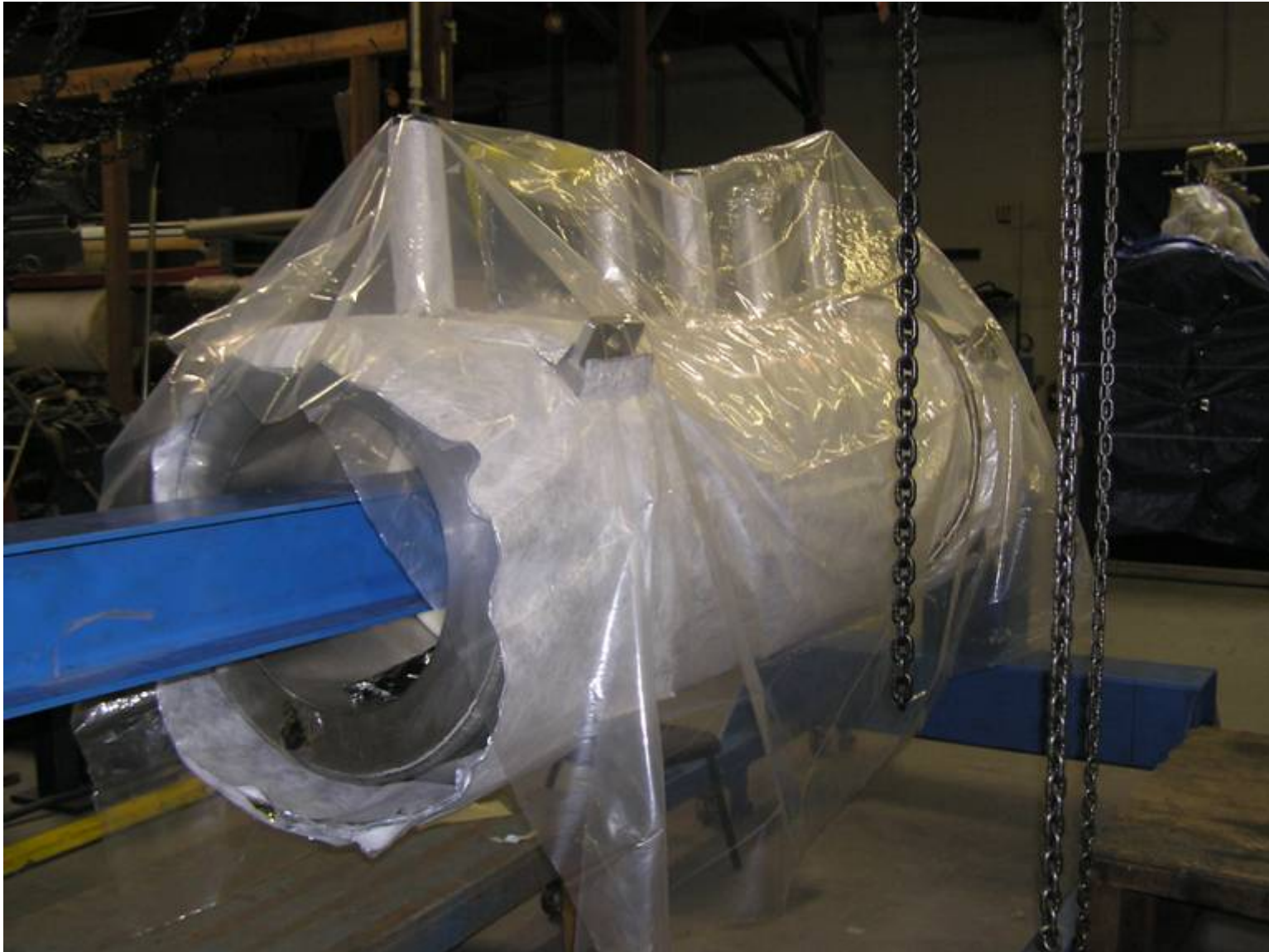
MLI wrapped cold mass in preparation for assembly into vacuum vessel (w/plastic cover)
