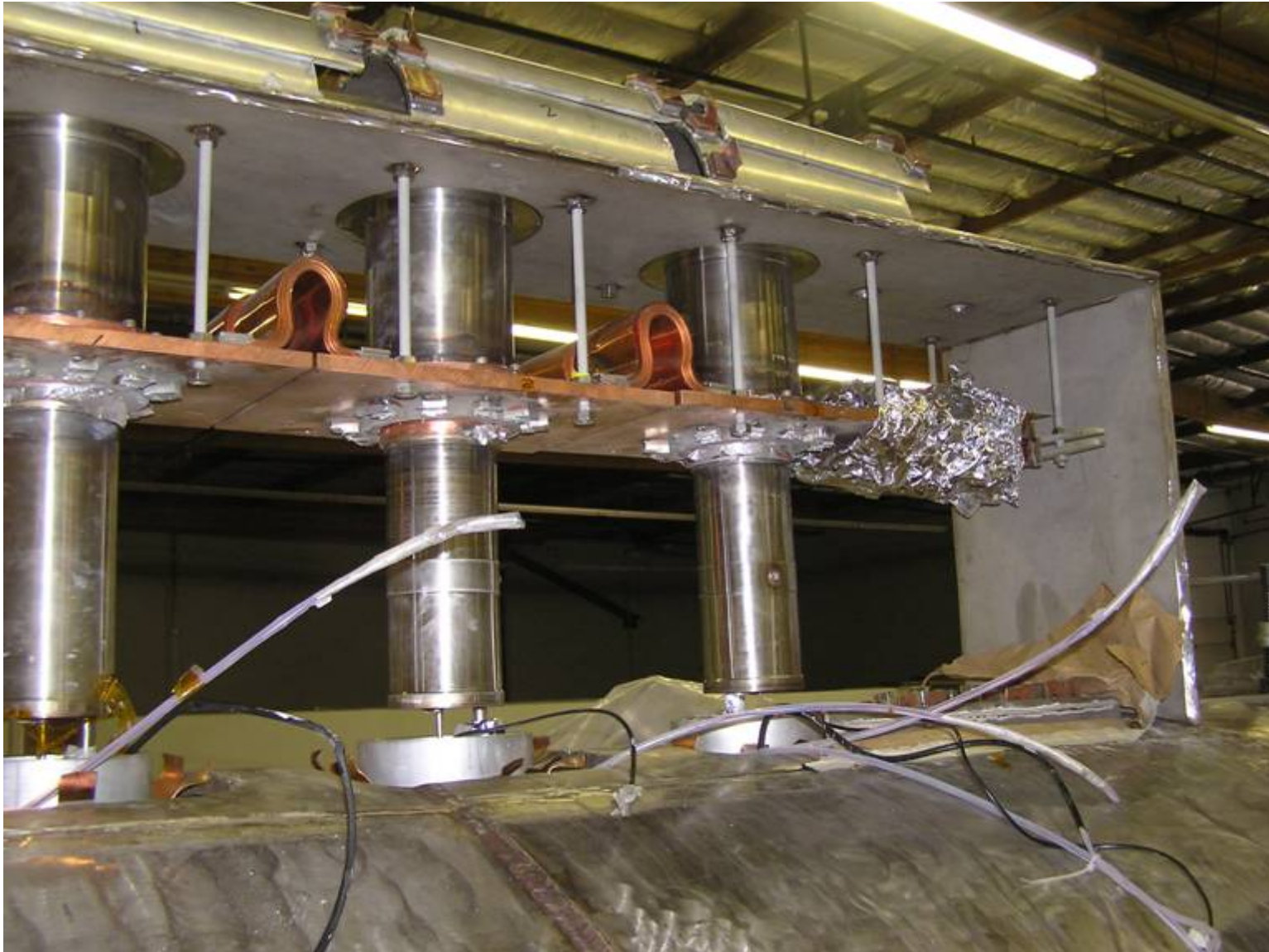
Cryocooler sleeves and 1 st stage copper plate (Magnet 1)
