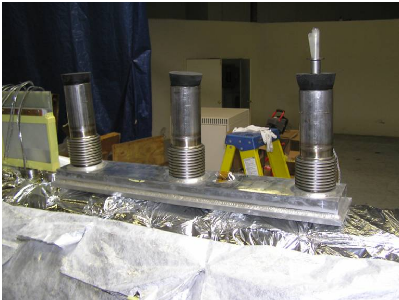
Cryocooler port manifold and connection sleeves/bellows
