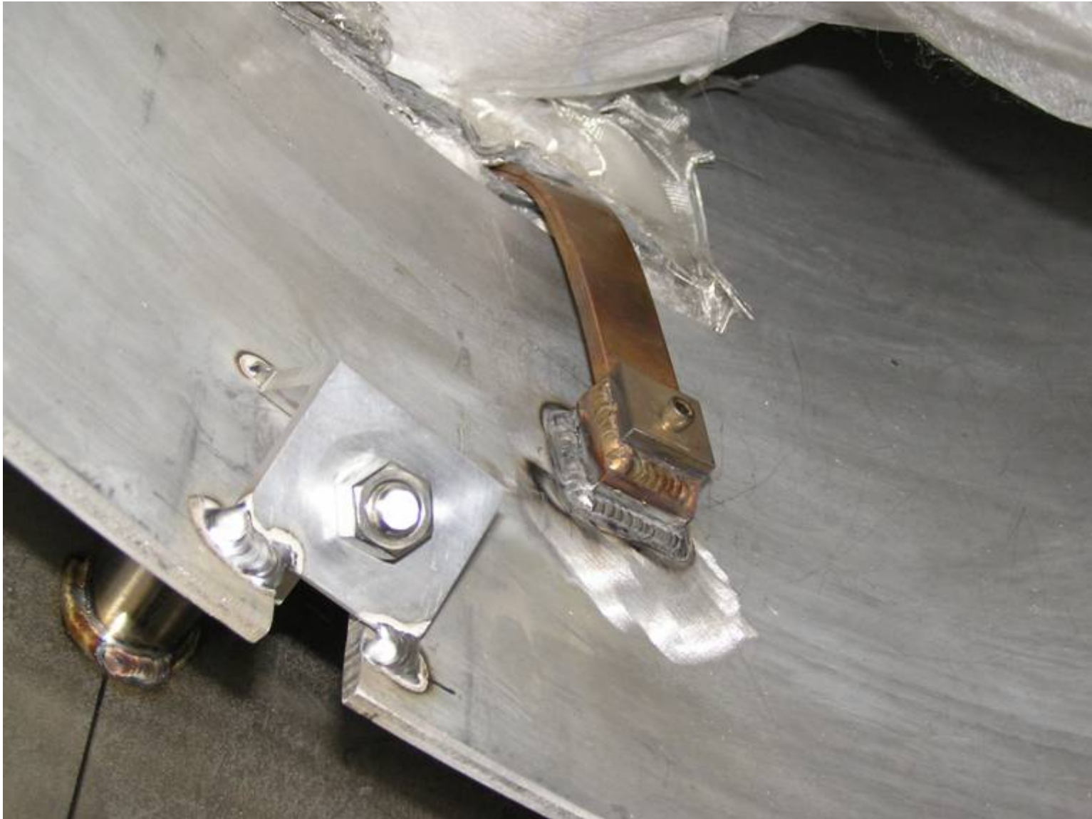
Cold mass support copper strap connection and thermal shield support mount
