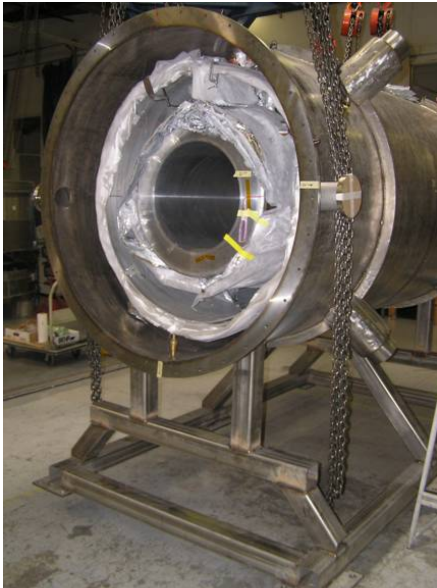
Alignment of cold mass in preparation for end plate installation
