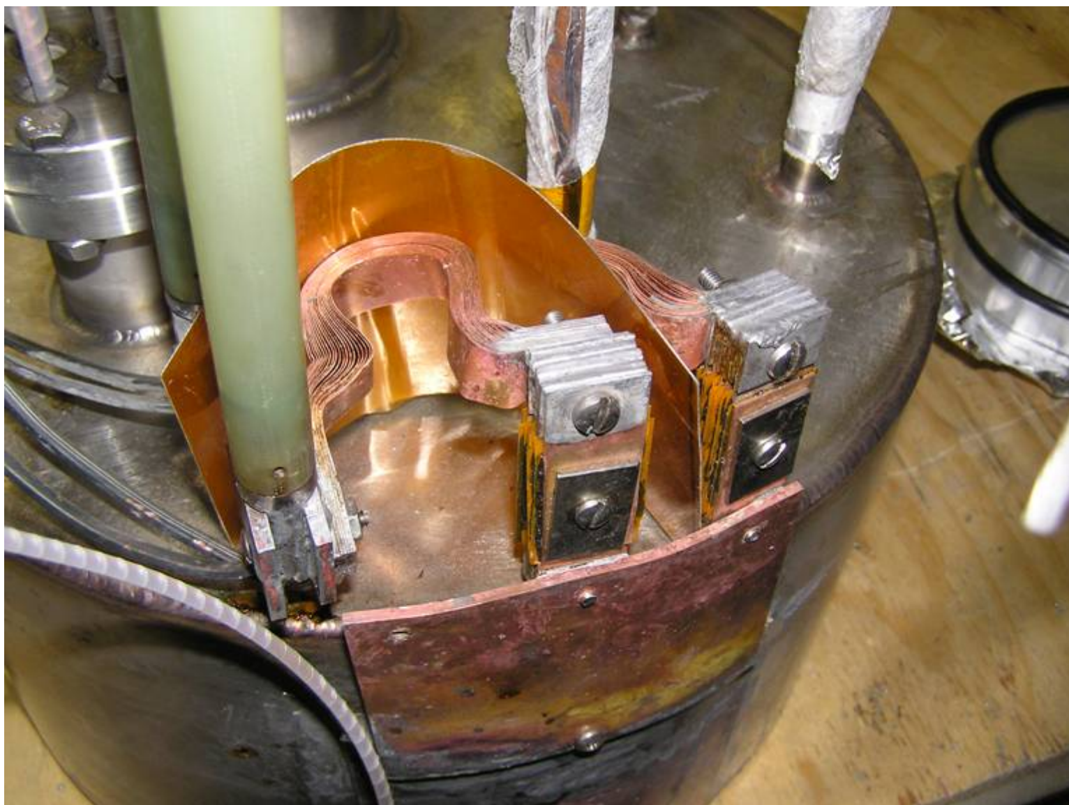
Thermal intercept to He vessel (cold mass) at lower end of HTS leads
