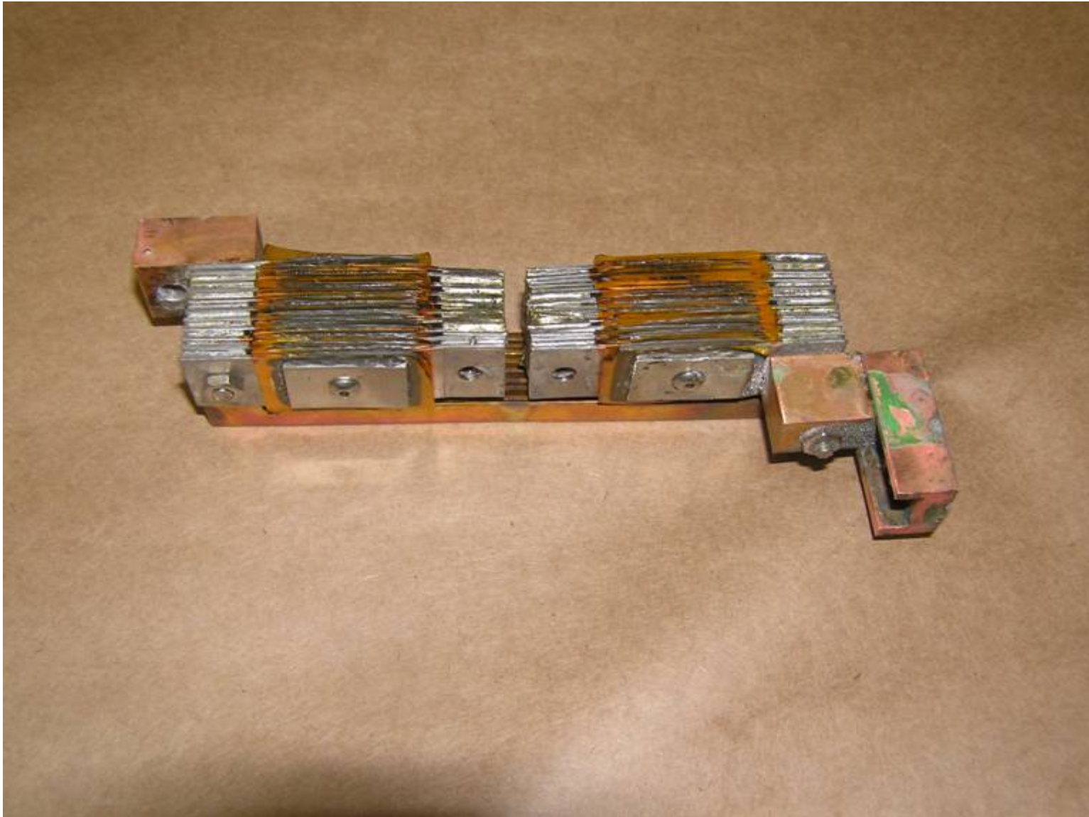
Thermal intercept assembly for connecting upper HTS leads and 1 st stage cooler plate
