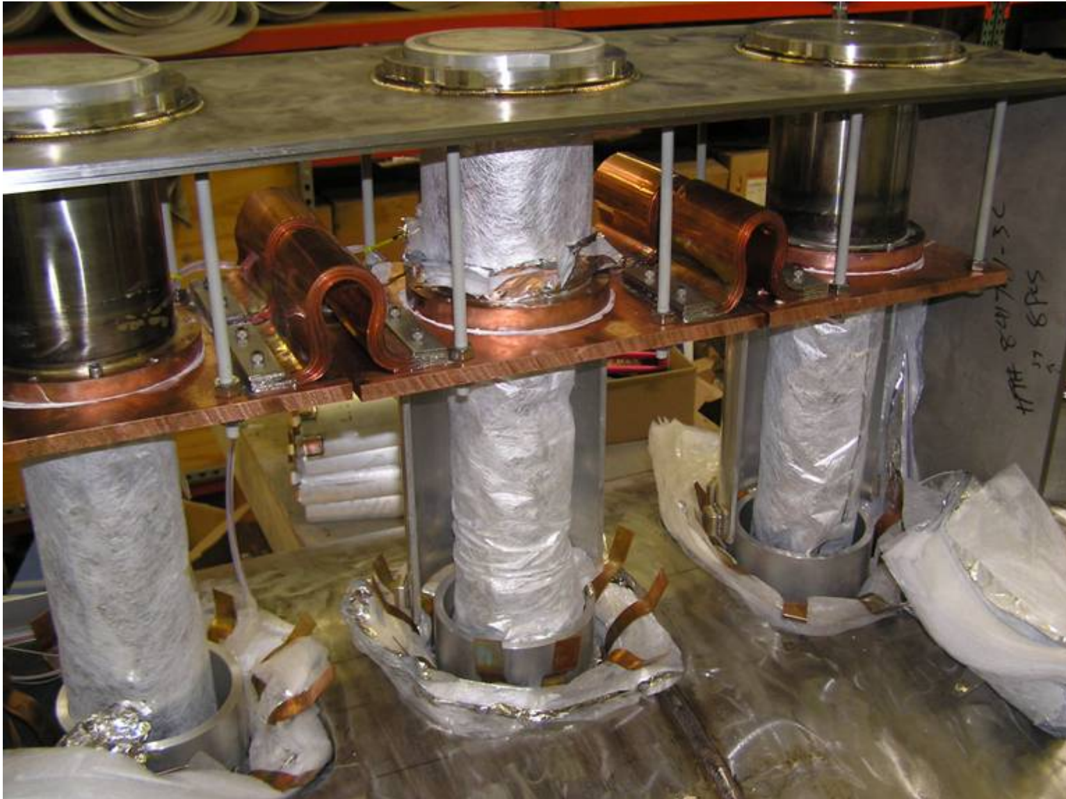
Cryocooler sleeves with 1 st stage connection to shield being assembled (Magnet 1)
