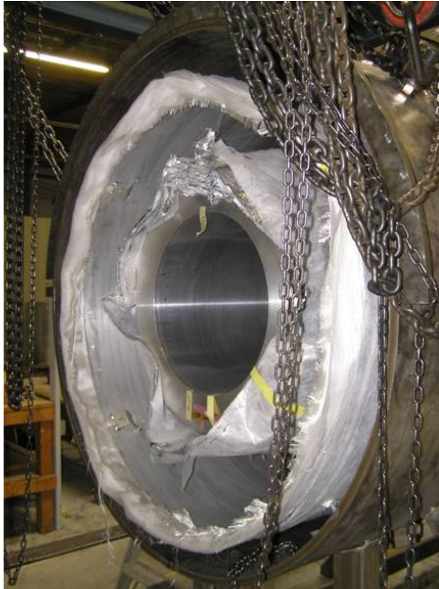
MLI wrapping on thermal shield and cold mass
