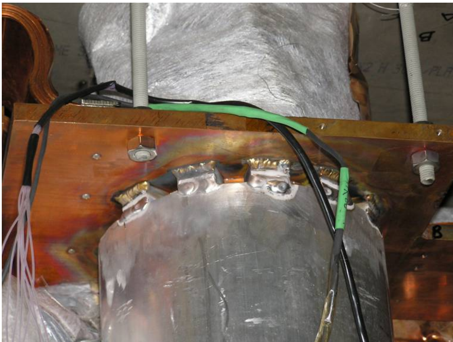
Upper end of cryocooler sleeve attachment to 1 st stage copper plate
