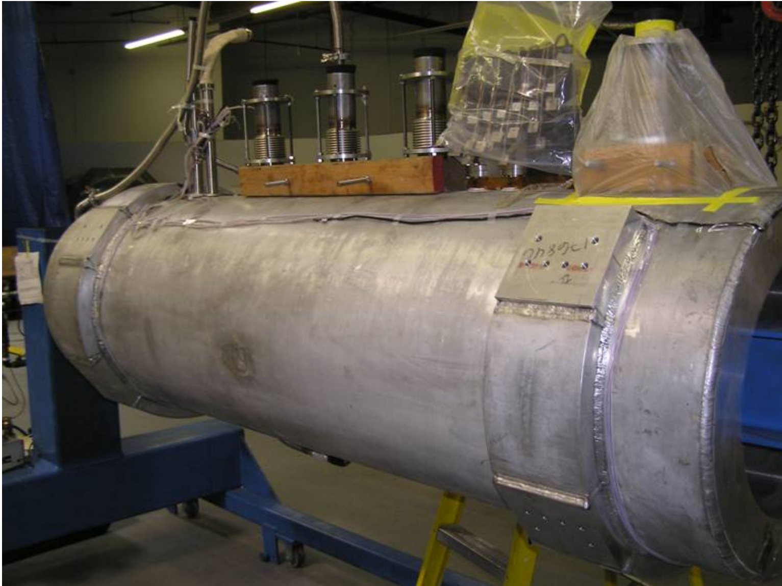
Final leak check of Magnet 1 cold mass assembly (2 nd iteration)
