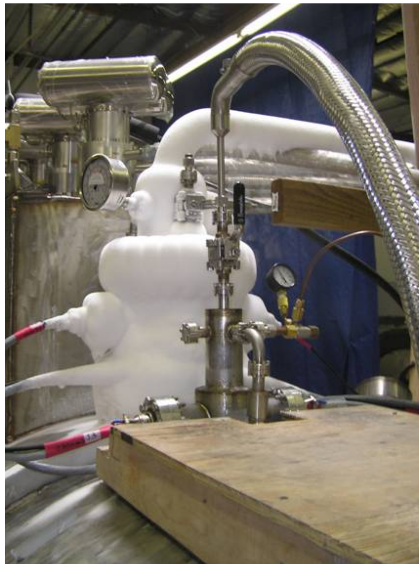
Magnet cooldown using liquid helium (Magnet 2)
