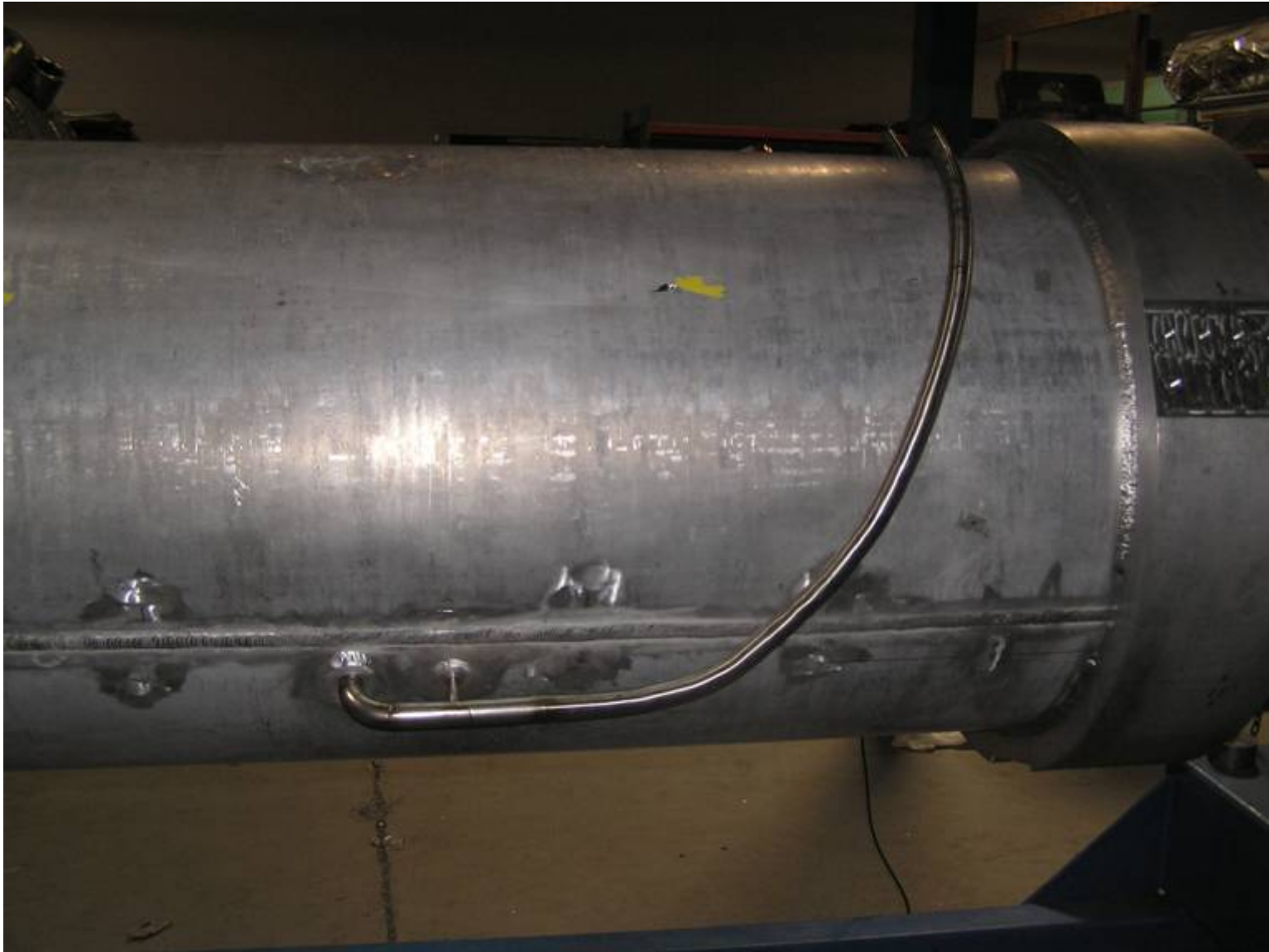
Newly configured cryogen fill tube for Magnet 1 (90° bends eliminated)
