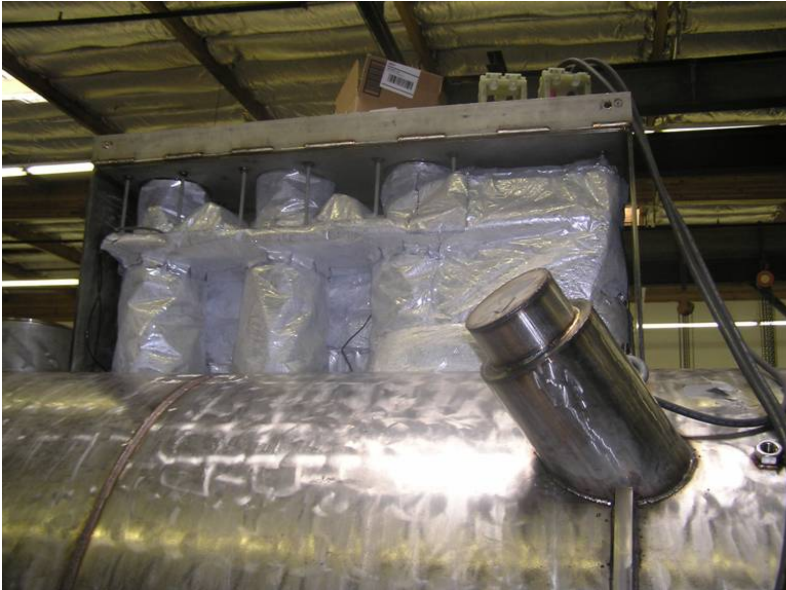
MLI wrapped cryocooler sleeves and magnet leads in turret area
