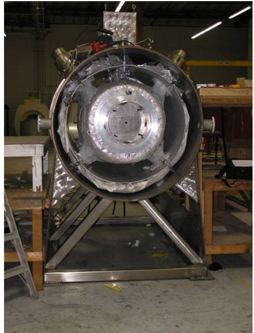
Alignment of cold mass in preparation for end plate installation
