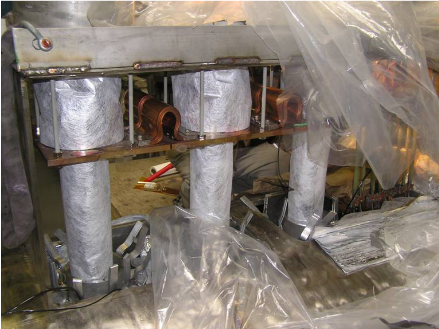
Cryocooler sleeves with MLI wrapping (Magnet 2)
