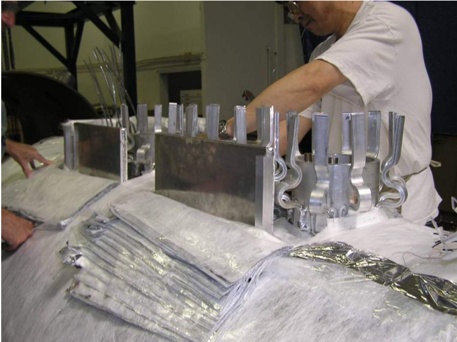
MLI wrapped shield with cryocooler 1 st stage connections and plates welded to shield for LN reservoir attachment (Magnet 2)
