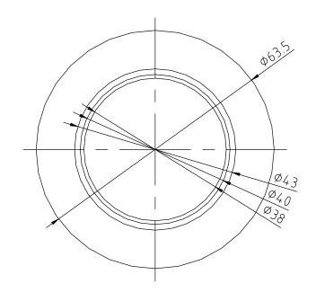
NAME: VALVE INSTALL TUBE PLATE
