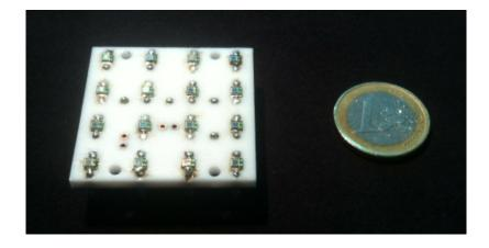
**Figure 11.** Dice Board, used in NEXT-DEMO, containing 16  $(4\times4)$  MPPCs.
