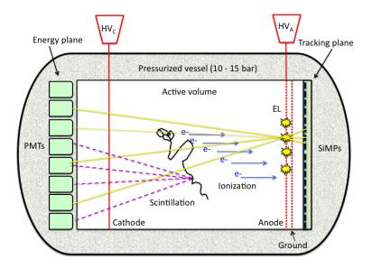
**Figure 2.** The *Separate*, *Optimized Functions* (SOFT) concept in the NEXT experiment: EL light generated at the anode is recorded in the photosensor plane right behind it and used for tracking; it is also recorded in the photosensor plane behind the transparent cathode and used for a precise energy measurement.
