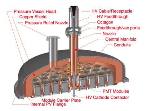
**Figure 15.** The full energy plane of NEXT-100 mounted in the vessel head.
