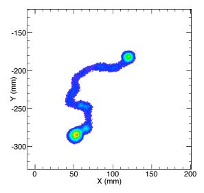
**Figure 1.** Monte-Carlo simulation of a  $^{136}$ Xe  $\beta\beta0\nu$  event in xenon gas at 10 bar: the ionization track, about 30 cm long, is tortuous because of multiple scattering, and has larger depositions or *blobs* in both ends.
