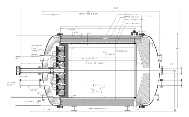
Figure 7. Pressure Vessel/Detector: side cross section view.
