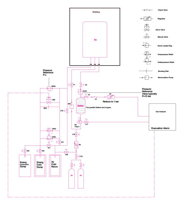
Figure 19. Schematic of the NEXT-100 gas system.
