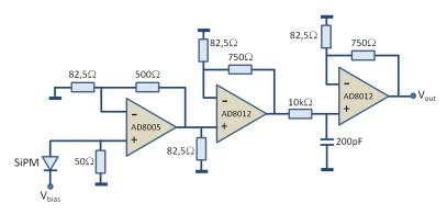
**Figure 17.** This low power amplifier circuit for NEXT-100 features only 30 mW power, 4 mV/pe gain and 1.7 mV rms noise.
