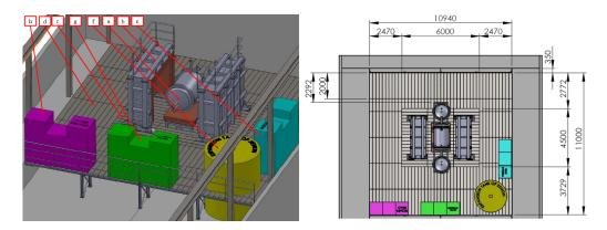
**Figure 21.** Left: Intended location of the components and subsystems for the operation of NEXT-100 on the working platform: (a) NEXT-100; (b) the lead castle shield in its open configuration; (c) seismic platform; (d) working platform; (e) gas purification system; (f) emergency gas vent tank; (g) data acquisition system; (h) other systems. Right: Top view showing the dimensions of the working platform.
