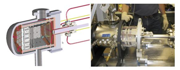
**Figure 3.** The NEXT-DBDM prototype, operating at LBNL. Left: cross section of the detector. Right: insertion of the time projection chamber into the stainless-steel pressure vessel.
