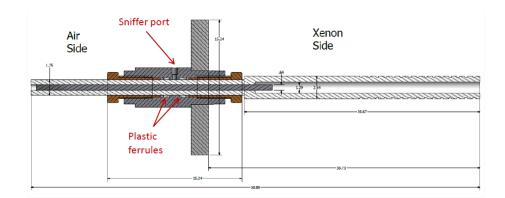
Figure 9. Cathode high-voltage feedthrough (HVFT) designed for operation up to 100 kV.
