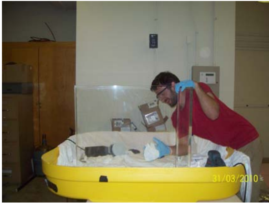
Figure 2.17: (Color online) A piece of scintillator in its final polishing stage, hand buffing with an antistatic cream.
