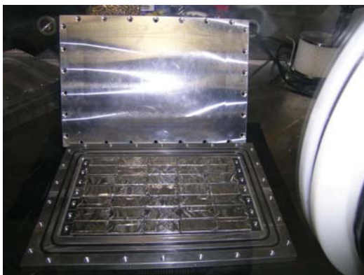
Figure 9.33: (Color online) A photograph of the rubidium intercalated graphite monochromator assembly prior to installation.
