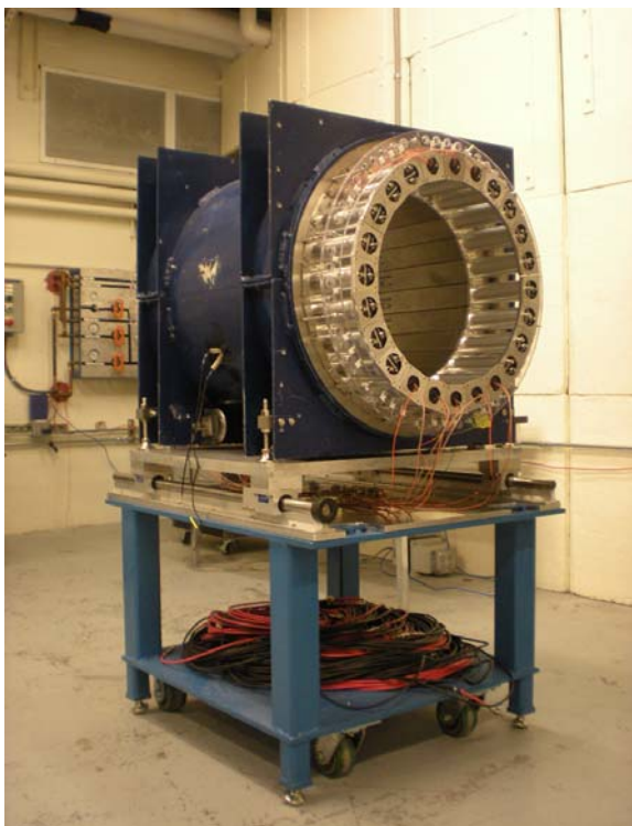
Figure 9.24: (Color online) Photograph of the fully constructed APEX detector outfitted with 48 new PMTs and aluminum mounts.
