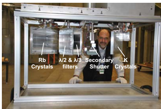
Figure 9.34: (Color online) A photograph of the complete monochromator and filter assembly prior to installation.
