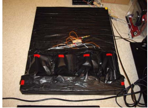
Figure 2.18: (Color online) A fully polished and wrapped piece of scintillator.
