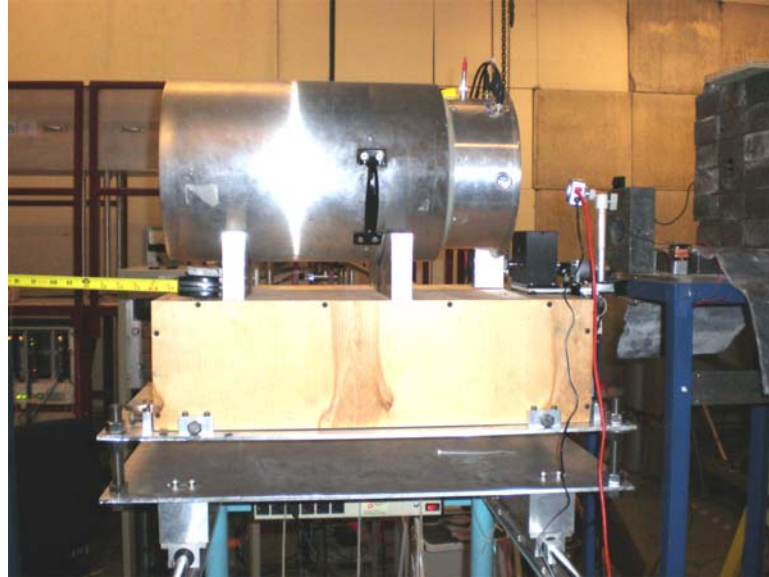
Figure 9.13: Photograph of the INVS counter. A large cylindrical polyethylene body envelops 18 ^3\text{He} proportional-counting tubes, each containing 6 atm of ^3\text{He} . Maximum detection efficiency for this detector is \sim 64\% .
