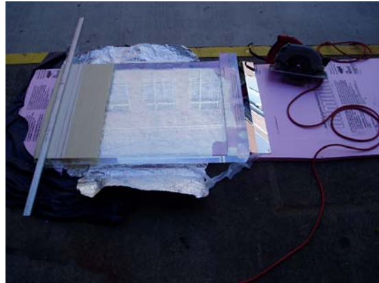
Figure 2.16: (Color online) A piece of scintillator right before it was cut. Masking tape covers the area being cut to help protect the scintillator from being further scratched and so that a line could be drawn to help guide the saw.
