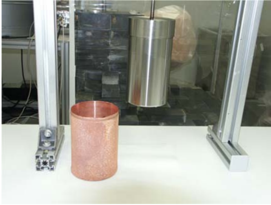
Figure 2.1: A copper piece that the collaboration electroformed underground at the Waste Isolation Pilot Plant in Carlsbad, NM in 2007. The mandrel used is also visible. The pieces that will be electroformed at the CETC will be similar, but larger.
