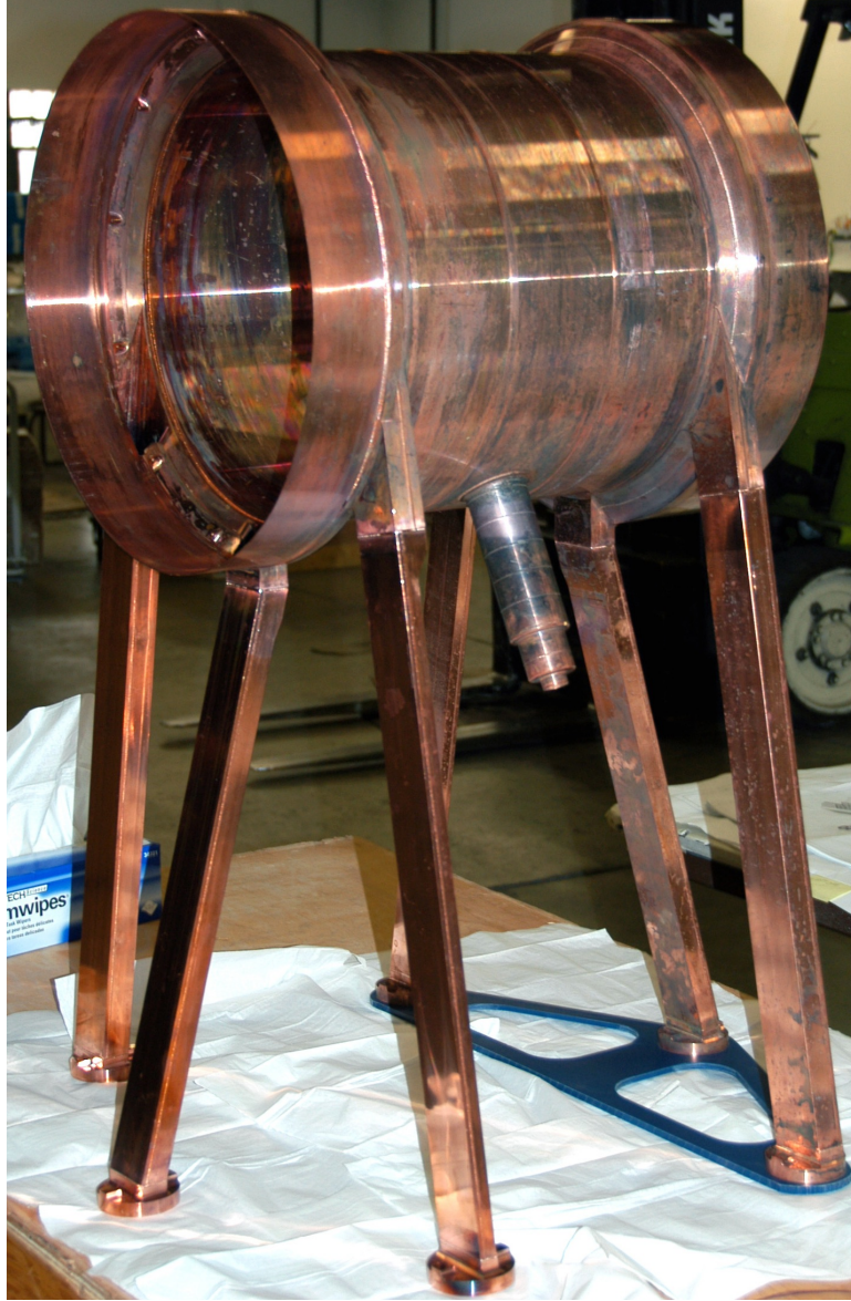
Figure 19. The completed LXe vessel before etching and welding to the cold hatch of the cryostat.
