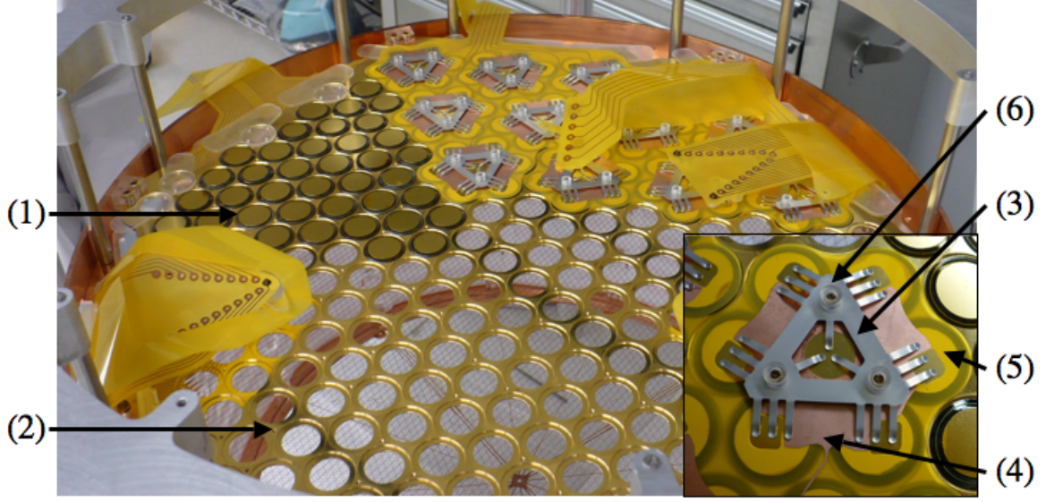
Figure 5. Bare LAAPDs are placed in a sector (1) of one platter (2). The platter is gold coated on this side for improved electrical contact. Platinum plated photo etched phosphor bronze “spider” springs (3) anchor gangs of 7 LAAPDs to the copper platter, and provide electrical contact between the cathodes of each LAAPD and copper traces (4) on flexible cables (5), as shown in the inset. Acrylic washers (6) prevent electrical contact between the springs and the mounting screws that are threaded into the platter. Ionization-collecting wires (and the cathode grid) can be seen through the partially filled LAAPD platter (7).
