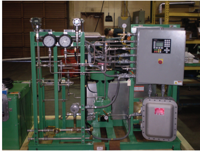
Figure 7.10: Example of the re-circulation pump chosen for the Xe purification gas system. This is a triple stainless steel diaphragm pump capable of 100 slpm flow rates.
