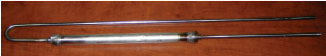
Figure 7.8: ^{222}\text{Rn} trap operated at SNO lab. The trap uses activated carbon spheres to slow transmission of radon atoms. The trap tested on removing Rn from Ar gas and operates at a -110^\circ\text{C} .
