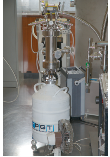
Figure 7.17: Photograph of the ZEPLIN III electron lifetime monitor positioned on the liquid nitrogen cryostat.
