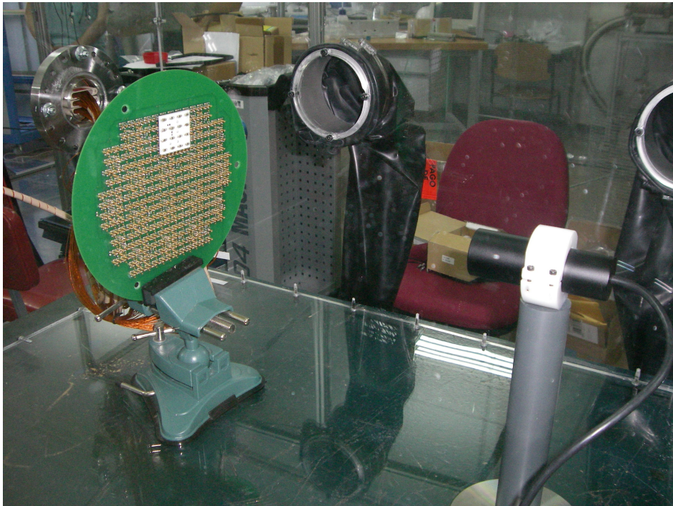
Figure 4.14: PMT Tracking plane installed at the TPC Anode in the commissioning of NEXT1 operation.
