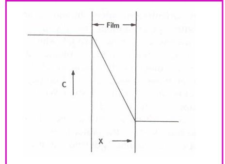
Schematic of steady state diffusion
