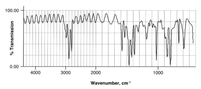
Figure 6. Infrared Transmission Spectra of Parylene N
