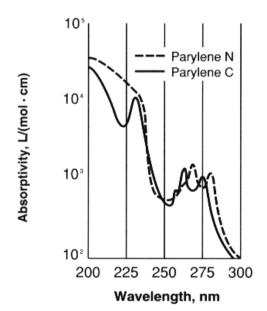
Figure 4. Ultraviolet Absorption Spectra of Parylene N and C
