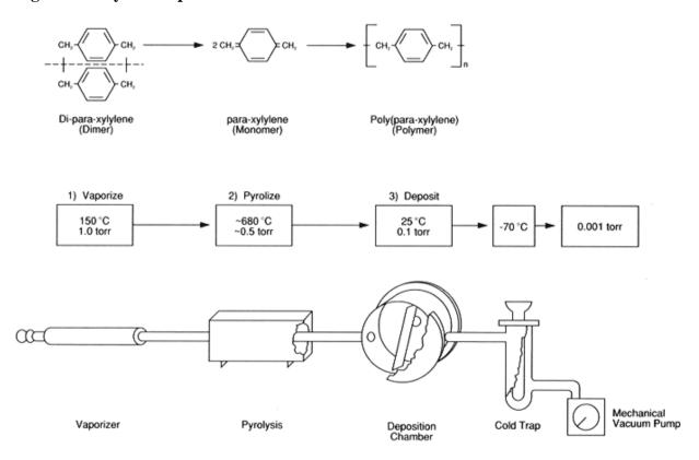
The equipment can be modified to meet the requirements or configuration of the items to be coated. Present coating chambers vary in size from 23 cm in diameter and 31 cm long to a 85 cm high hemi-cylindrical unit. One particular configuration, 45 cm in diameter and 60 cm high, was designed specifically for circuit boards and can accommodate up to two hundred 12 cm wide by 16 cm long boards. The process is inherently simple and can be conducted with a minimum of supervision.
