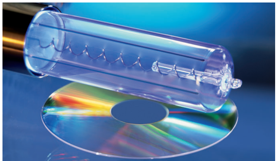
Irradiation of glass substrates for improving wettability before deposition of magnetic layers.
