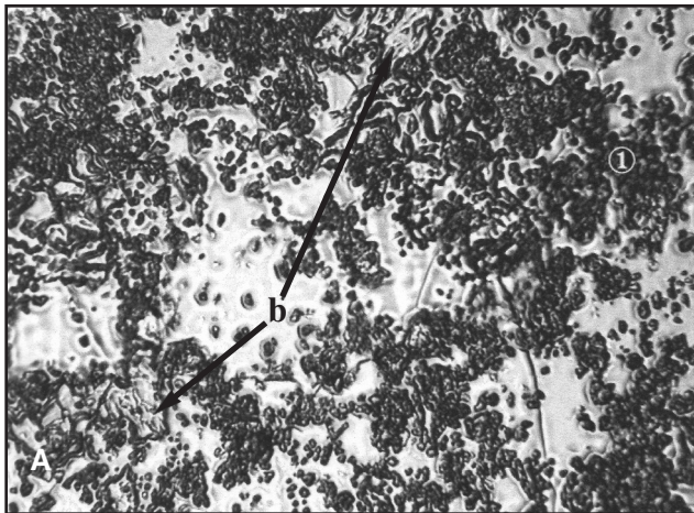
Fig. 6 — Optical micrographs of the fracture surface from an unpolished diffusion bond that failed at 48 MPa, showing matching regions of (A) metal and (B) ceramic sides. The region labeled 1 is deformed metal. The regions marked “b” indicate bonded regions; regions marked “c” indicate the presence of silicides.
