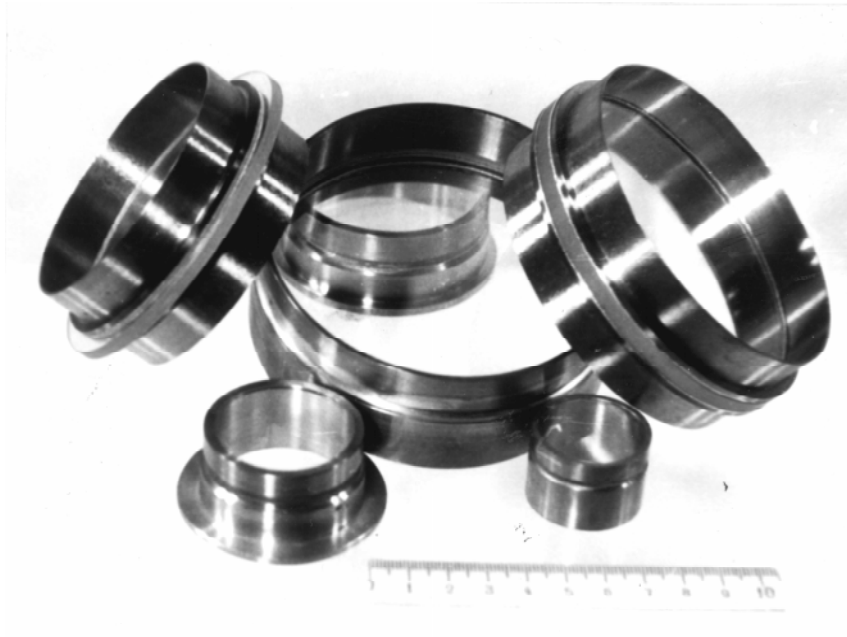
Fig. 2. Bulky diffusion bonded and brazed titanium-to-sapphire windows.
