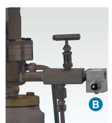
Since the set pressure of all modulating safety valves in this catalogue are defined as the point when the dome pressure is reduced to 70 percent of set pressure, when system pressure reaches the nameplate setting, the indicator is activated. This gives positive verification that set pressure has been reached. The verification process for modulating pilots requires this option, in addition to the Field Test Connection.
