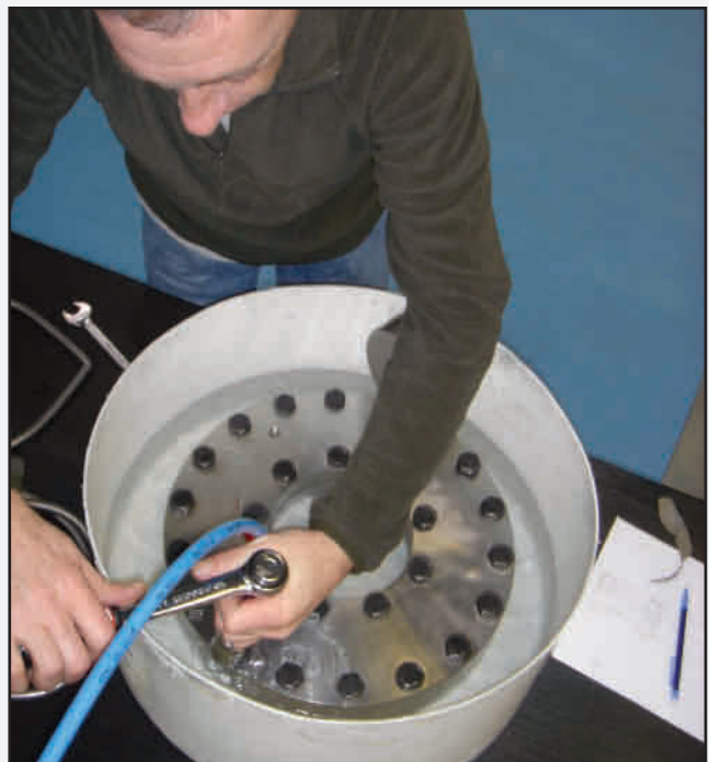
Tailor made leaktest
