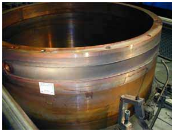
Source: TWI Copper canister for storage of High Level Waste (nuclear), for SKB Wall thickness: 50 mm!
