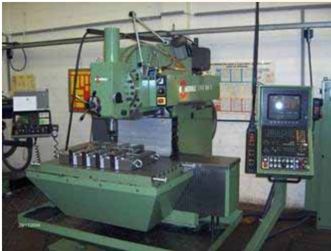
Source: UCL-PRM Milling machine adapted for FSW
