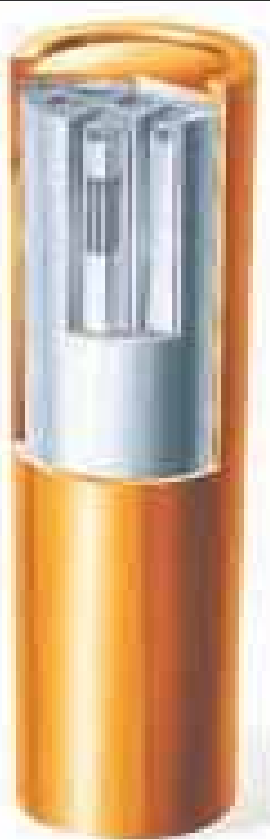
Source: TWI Copper canister for storage of High Level Waste (nuclear), for SKB Wall thickness: 50 mm!
