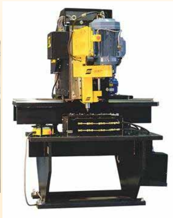
Source: ESAB (Legio) Small FSW machine
