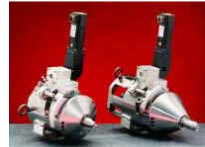
Self-retractable pin tool Source: NASA
