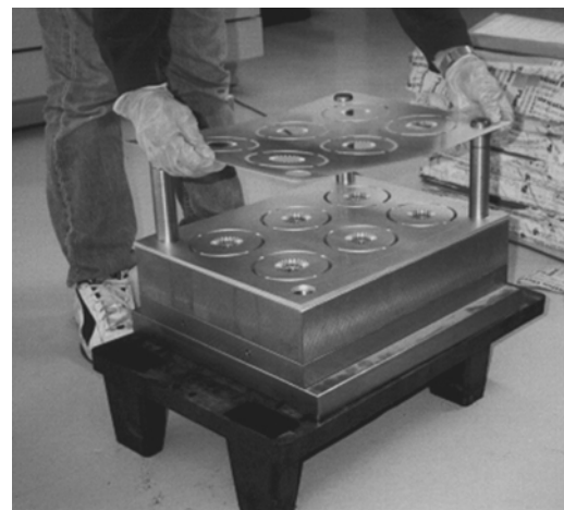
Fig. 6.9 Patterned, plated, and stacked sheets, aligned in a jig ready for application of the compressive load and diffusion brazing in a vacuum oven. The diffusion brazing conditions were a compressive stress of 3 MPa (440 psi) and a process temperature of 820^\circ\text{C} ( 1510^\circ\text{F} ), sustained for 10 h.
