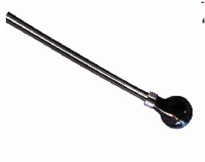
Example of T sensor permanent attachment with Stycast
