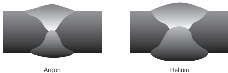
Figure 36 – Effect of argon and helium shielding gases on weld profile when welding aluminum (DCEP)
