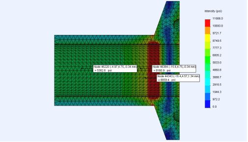
**Inside General stress**: The stress display has been capped off at the Primary Membrane allowable stress of 11,666 PSI. The highest general stress on the inside face is shown above to be 8,859 PSI, which is acceptable because it is less than the Pm limit noted above. Inside General Stress is acceptable
