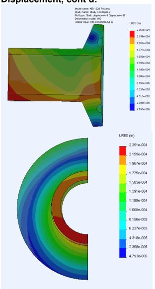
The resultant ferrule displacement is displayed in the figures to the left. The display has been capped at 2.351E-4 in, so that the colour bands could be differentiated. The clamp has been hidden both for clarity and because it is excluded from this analysis as it is already CRN approved.
