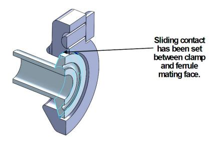
**Sliding Surface:** A sliding surface condition was applied at the touching surfaces of the clamp with the ferrule's flange.
