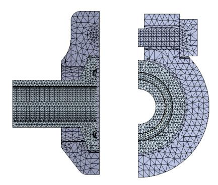
The figures above show the mesh sizes used. The Mesh characteristics are:
