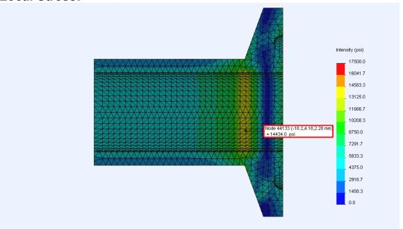
Inside Local stress: The stress display has been capped off at the Local Membrane+ Bending (PI+Pb) allowable stress of 17,500 PSI. The highest Local Stress on the inside face is shown above to be 14,434 PSI, which is acceptable because it is less than the PI+Pb limit noted above. Inside Local Stress is acceptable
