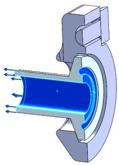
**System Pressure:** As shown above, a system pressure of 1,200 PSI was applied to all applicable internal faces. A pressure-equivalent force was applied to the end of the tube, as shown.
