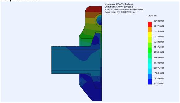
**Overall Displacement:** The figures above and below show the overall relative displacement as viewed from the inside and end, respectively. The peak relative displacement is 0.00095" as shown at the top of the clamp. The displacement in the flange is 0.00023". Color band differences between the flanges and clamp show that the sliding contact was properly applied. Displacement is Acceptable.
