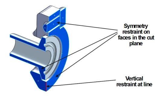
**Restraints**: The figure above shows the restraints that were used on the model. A symmetry constraint has been applied to the faces in the two cut-planes. A vertical restraint has been applied where shown.
