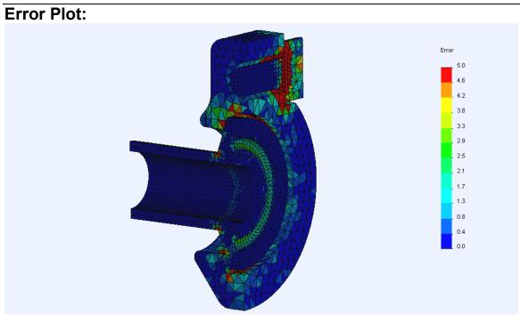
**Overall Error Plot**: The figure above shows that the error is <5% in all critical general areas of the Tri-Clamp ferrule. Areas with error over 5% are directly at the discontinuity and no more than one element away from it. Error plot is acceptable.
