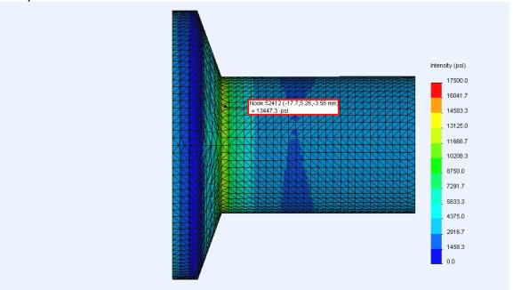
**Outside Local Stress:** The figure above shows the Outside LocalStress, with the display capped at the PI+Pb limit. The highest stress is 13,447 PSI, as shown above. It is acceptable because it is less than PI+Pb=17,500 PSI. Outside Local Stress is Acceptable.
