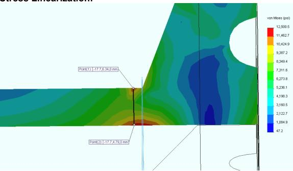
**Linearization:** For the cross-sectional area shown above, the membrane stress is 7,694 PSI, which is acceptable because it is less than the allowable Pm stress of 11,666 PSI. The highest PI+Pb (Local Membrane + Bending) stress is 11,821 PSI, which is less than the 1.5\*kS limit of 17,500 PSI. Stress is acceptable.
