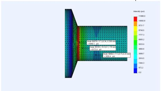
**Outside General Stress:** The figure above shows the Outside General Stress, with the display capped at the Pm limit. The highest general Primary stress is 8,040 PSI, as shown above. It is acceptable because it is less than Pm=11,666 PSI. General Outside Stress is Acceptable.
