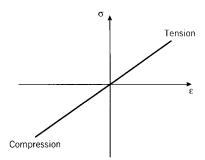
Figure 15: Stress-strain curve in tension and compression.
