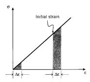
Figure 12: Energy associated with increments of strain
