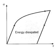
Figure 14: Energy loss = area under stress-strain loop.
