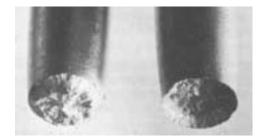
Figure 5: Cup-and-cone fracture in a ductile metal.
