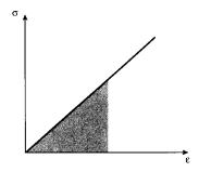
Figure 11: Strain energy = area under stress-strain curve.
