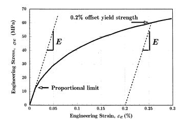
Figure 2: Low-strain region of the engineering stress-strain curve for annealed polycrystaline copper; this curve is typical of that of many ductile metals.
