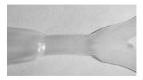
Figure 7: Necking and drawing in a 6-pack holder.
