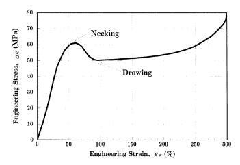
Figure 6: Stress-strain curve for polyamide (nylon) thermoplastic.
