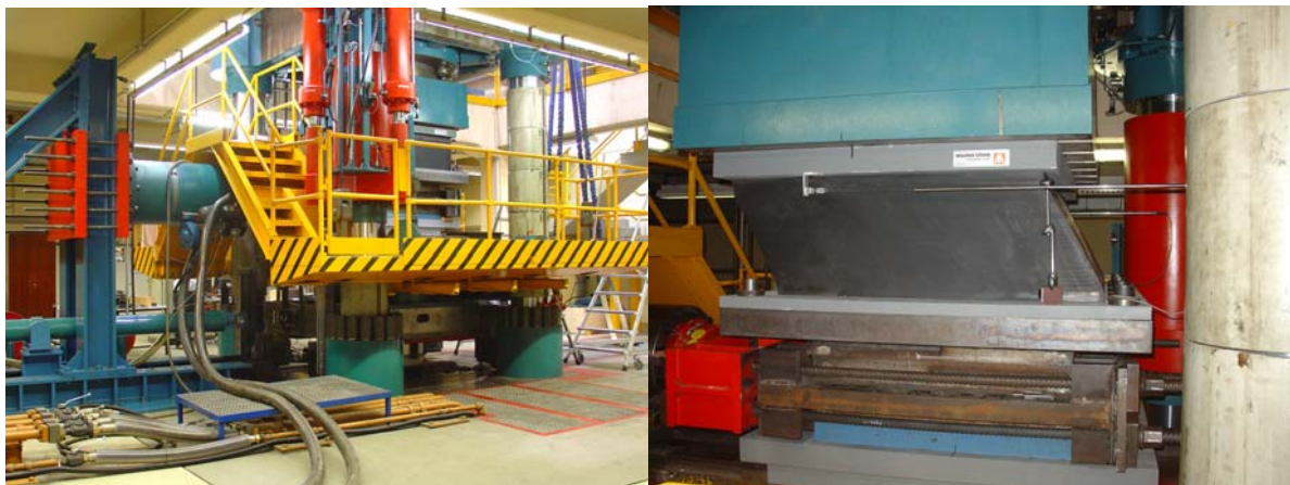
Fig. 16: Testing of a MLRB with 22.000 kN load in the testing rig of the University of Bochum
