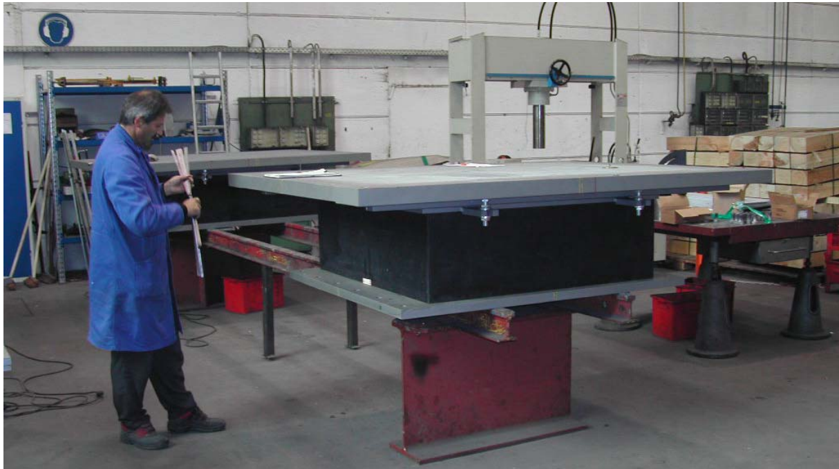
Fig. 15: Quality check after assembly of a MLRB with 1200 x 1200 x 440mm with lead core of 250mm diameter
