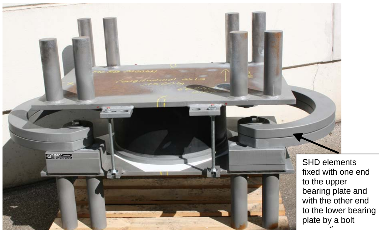
Fig. 18: MLRB isolator with SHD elements at both ends
