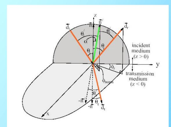
Coordinate system used for *ground* surfaces along with the definition of geometrical parameters.
