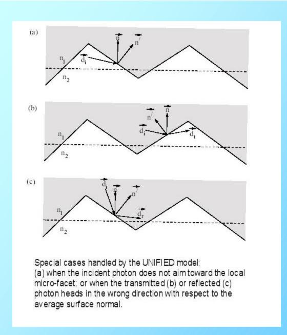
In cases (b) and (c), multiple interactions with the boundary are possible within the Process itself and without the need for relocation by the G4Navigator.
