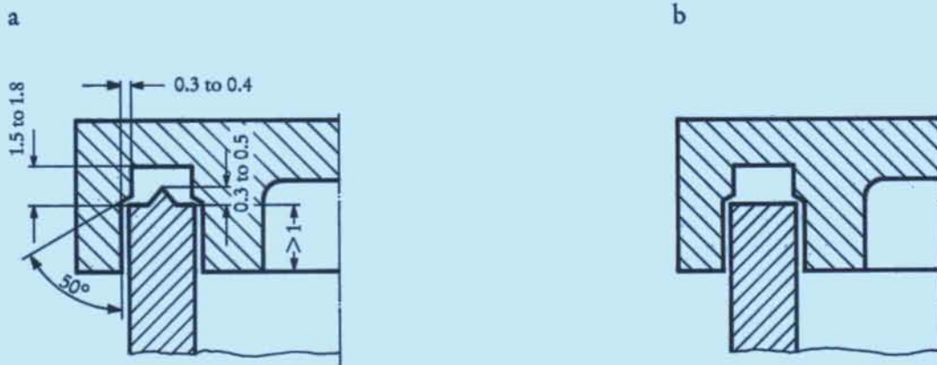
Fig. 22: Joint designs for double pinch welds (a) with and (b) without an energy director on the bottom part. Because of the high dimensional accuracy required, should preferably be used only for parts made to close dimensional tolerances.
