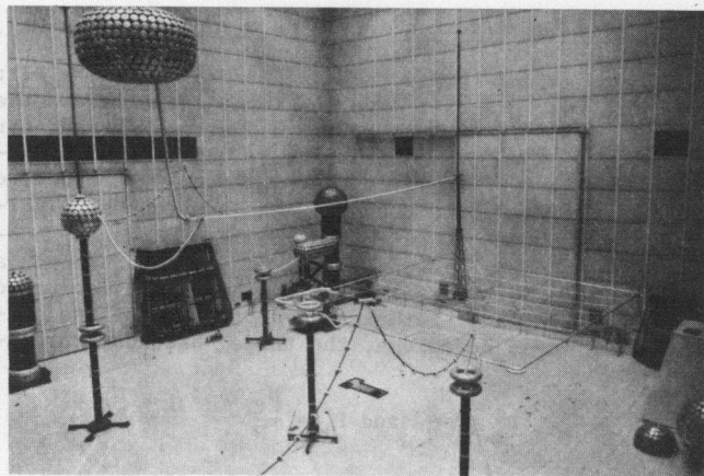
Fig. 3 Photograph of the setup for testing for the influence of the terminating electrodes.
