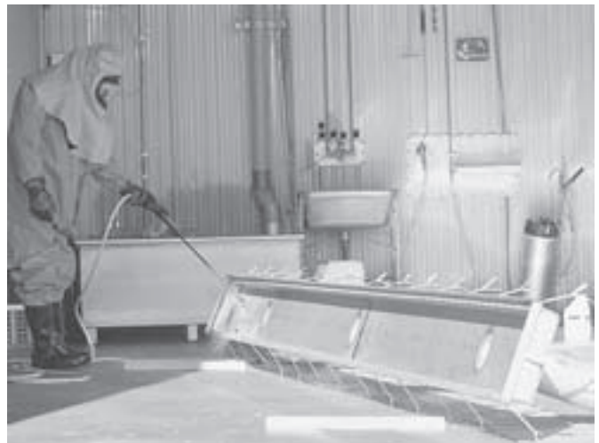
Figure 3. Application of Avesta Spray Pickle Gel
