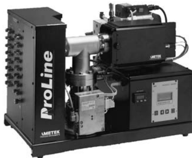
Figure 16: The ProLine Process Mass Spectrometer is capable of monitoring up to 16 gas lines for contamination and leakages at ppb level. In an event of detected leakage of ^{136}\text{Xe} an automatic gas evacuation procedure could be implemented. Additionally continuous monitoring for ^{222}\text{Rn} in the ^{136}\text{Xe} can be performed.
