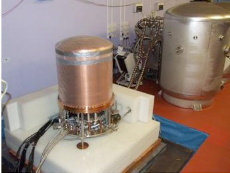
Figure 13: Example of an expansion tank that can be used for reducing the pressure in the NEXT 100 detector in an event of breach. One of the expansion tanks, from a set of two, used for ZEPLIN II and III is seen on the far background right.
