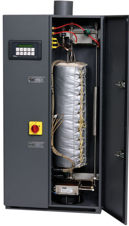
Figure 9: Example of a heated SAES getter model number PS4-MT50 with nominal flow of 150 slpm. This is a possible future upgrade to the gas system. The hot getter has been reported to be better at filtering out ^{222}\text{Rn} and therefore can be preferred purification technology to achieve ultra low radiation background rates.
