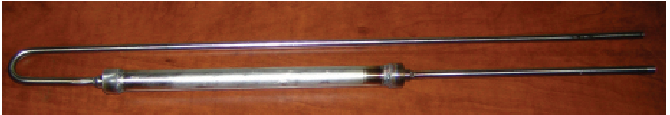
Figure 10: ^{222}\text{Rn} trap operated at SNO lab. The trap uses activated carbon spheres to slow transmission of radon atoms. The trap tested on removing Rn from Ar gas and operates at a -110^\circ\text{C} .
