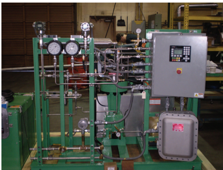
Figure 6: Example of the re-circulation pump chosen for the Xe purification gas system. This is a triple stainless steel diaphragm pump capable of 200 slpm flow rates.
