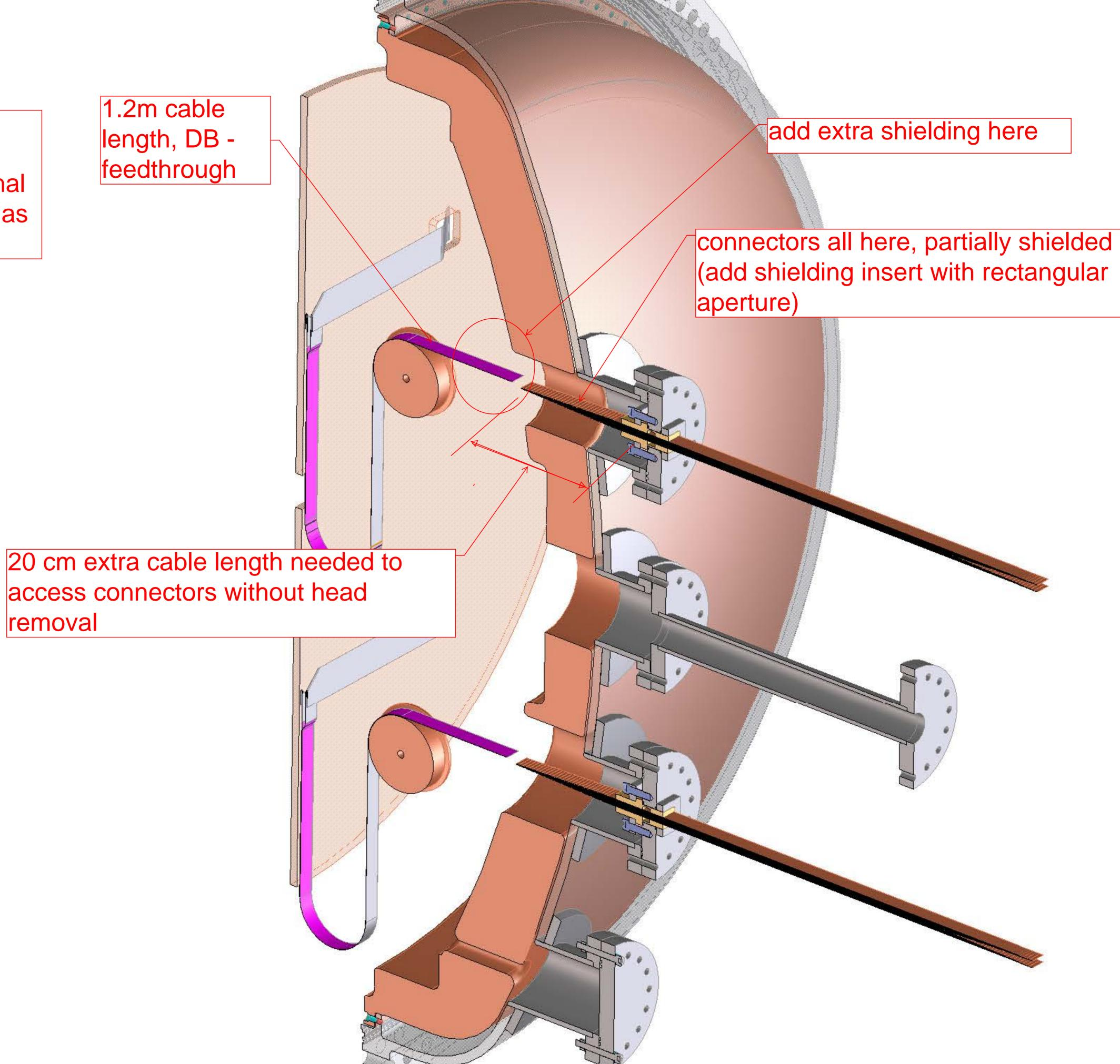
90 deg folds, 1mm radius; larger radii needed to avoid permanent set (which may be OK) will need clamps or "trays" to support horizontal cable runs may need supports here trunk will increase in thickness here, we will need to clamp this section down for support, just above the moving loops
