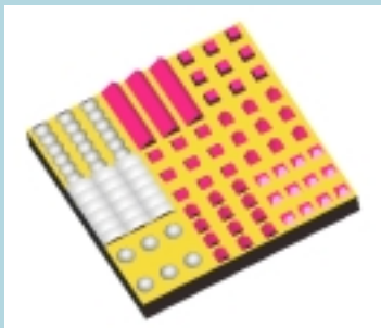
Figure 4 Texturing on lightguides is used with LCDs to diffuse the backlights. This lightguide shows some of the many patterns used on lightguides.
