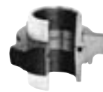
Fig. 300 Flat-Face Union 2,000 psi cwp - 3,000 psi test Size Range: 1" - 4"
