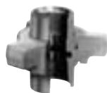
Fig. 607 Threaded Ends Well Service Union 2,000 psi cwp - 3,000 psi test Sizes: 1 1/2" & 2"
