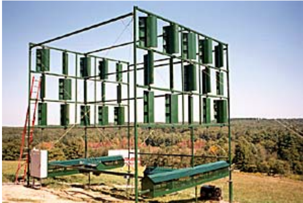
Figure 23: Mass Megawatts “Multi-Axis” Wind Turbine Prototype
