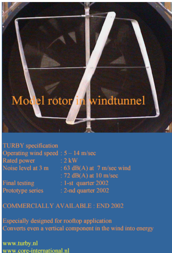
Figure 4.15. The Turby, with specifications
