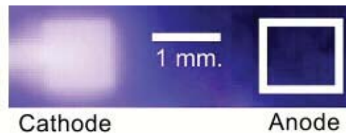
Fig. 1: Local confinement of a microplasma at 2 Torr and 410 V DC.
