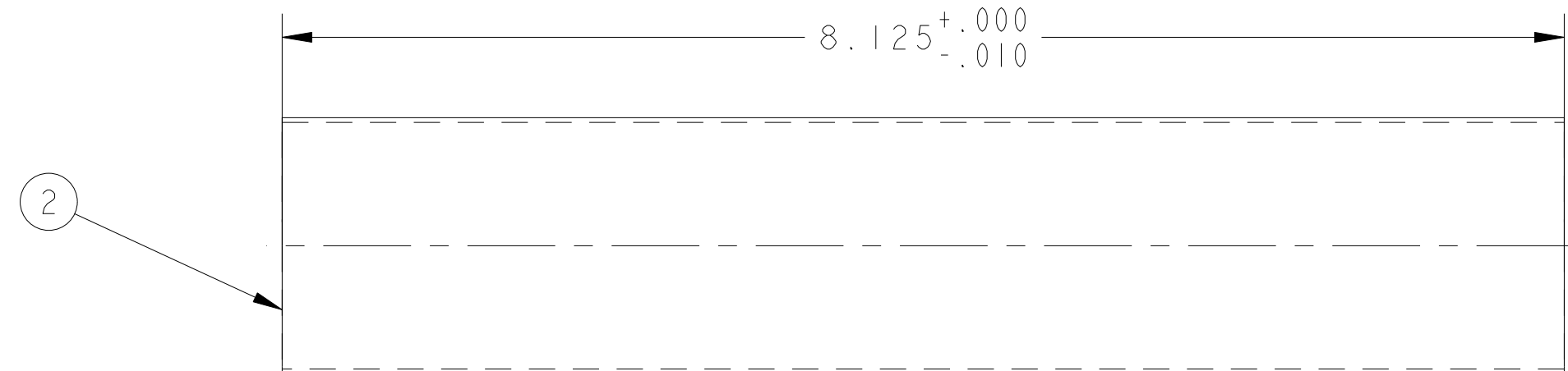
25B4774-05 BEAM PIPE 6
