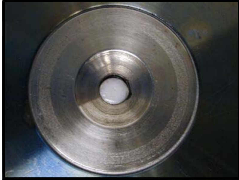
Figure 4.29. Displacement of an aluminosilicate source within the Pierce electrode after almost 220 hours of operation.
