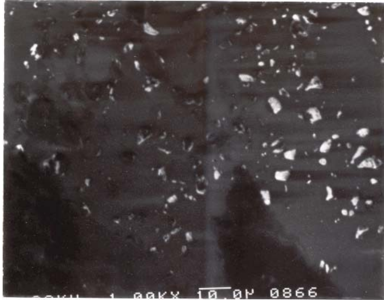
Figure 2.13. Photograph of the aluminosilicate prepared at 1,550°C. Note the aluminum oxide specs on the surface. 1,000X magnification.
