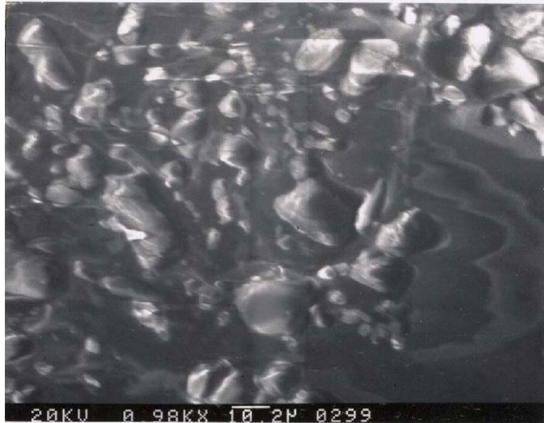
Figure 4.41 SEM photograph of the original appearance of the tested aluminosilicate emitter. The aluminosilicate is the glass-like smooth surface.
