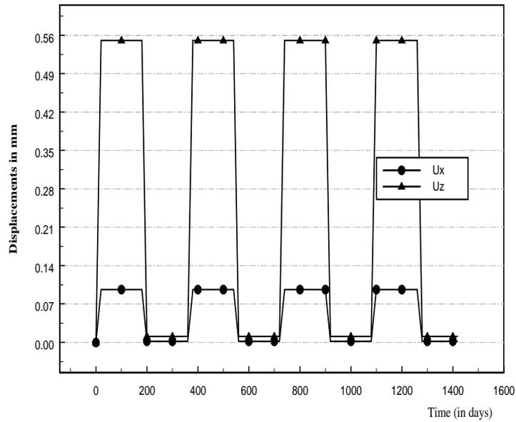
**Figure 13:** Time dependence on the  $U_x$  and  $U_z$  displacements, Carbon-Epoxy Hercules 3501-5,  $x/\text{thickness}=0$ ,  $(17, 17, 17, 17)_{SE}$  laminate,  $\Delta H = 0\%$ ,  $50\%$ .
