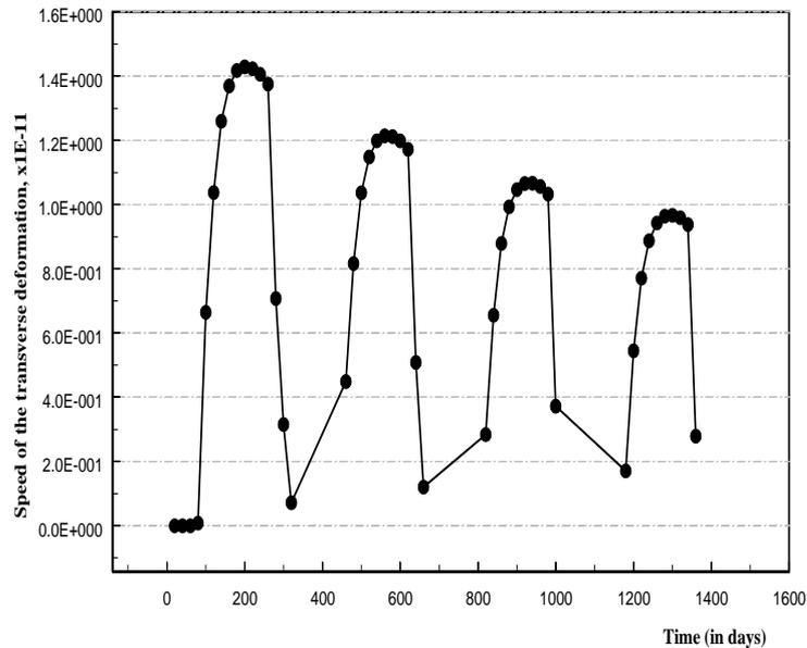
**Figure 10:** Time dependence on the speed of the transverse deformation, Carbon/Epoxy Hercules 3501-5,  $x/\text{épaisseur}=0.5$ ,  $\Delta H = 0\%$ , 50%.
