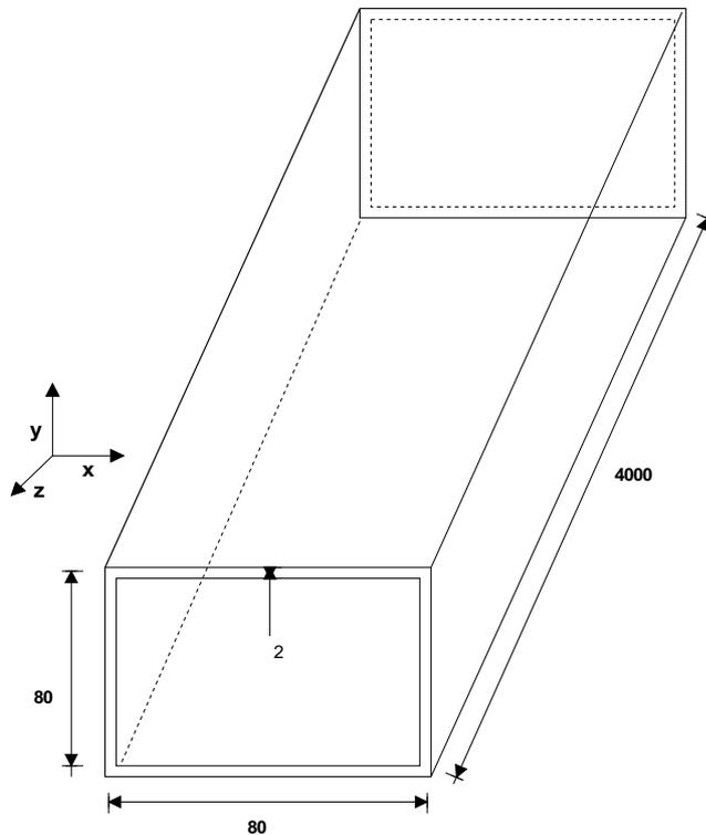
**Figure 1:** Dimensions in mm of the muon spectrometer alignment tubes
