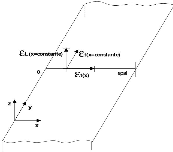
**Figure 5:** Hygroelastic deformations
