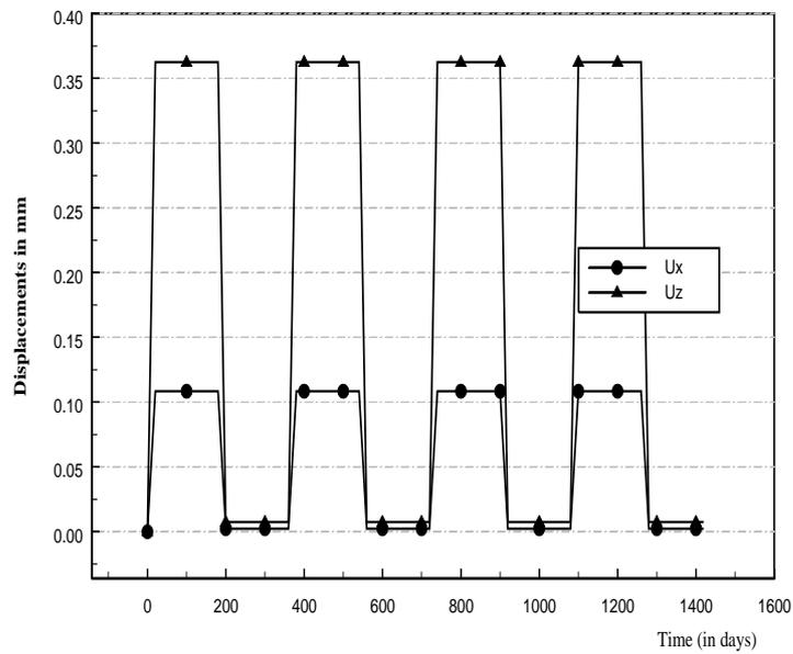
**Figure 12:** Time dependence on the  $U_x$  and  $U_z$  displacements, Carbon-Epoxy Hercules 3501-5,  $x/thickness=0$ ,  $(-10, 10, 0, 0)_{SE}$  laminate,  $\Delta H = 0\%$ , 50%.
