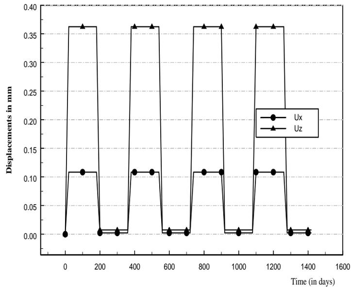
**Figure 11:** Time dependence on the  $U_x$  and  $U_z$  displacements, Carbon-Epoxy Hercules 3501-5,  $x/thickness=0$ ,  $(-15, 15, 0, 0)_{SE}$  laminate,  $\Delta H = 0\%$ , 50%.
