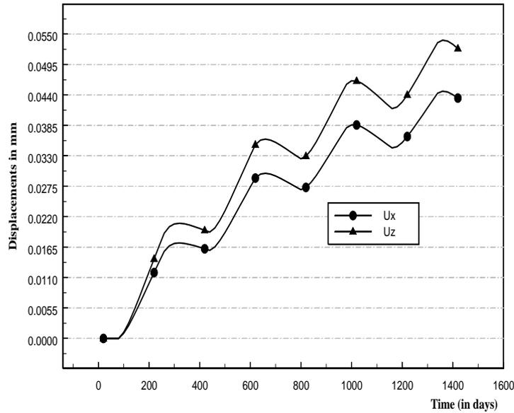
**Figure 9:** Time dependence on the displacements in mm, Carbon/Epoxy Hercules 3501-5,  $x/\text{thickness}=0.5$ ,  $\Delta H = 0\%$ , 50%.
