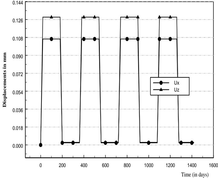
**Figure 8:** Time dependence on the  $U_x$  and  $U_z$  displacements, Carbon/Epoxy Hercules 3501-5,  $x/\text{thickness}=0$ ,  $\Delta H = 0\%$ , 50%.
