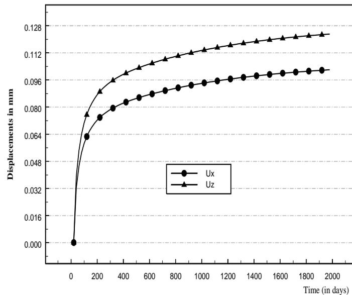
**Figure 7:** Time dependence on the  $U_x$  and  $U_z$  displacements, Carbon/Epoxy Hercule 3501-5,  $x/\text{thickness}=0.165$   $\Delta H = 50\%$ .
