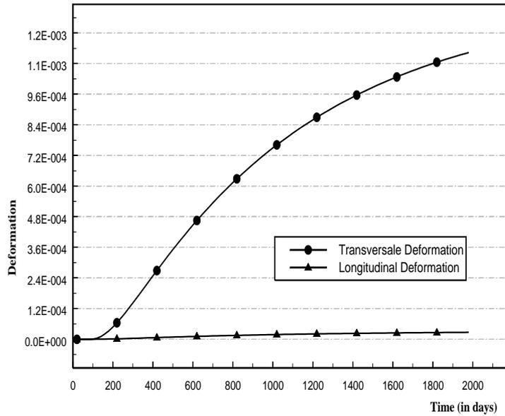
**Figure 2:** Time dependence on the hydroelastic deformations -Carbon resin epoxy Hercules 3501-5,  $x/thickness=0.5$ ,  $\Delta H = 50\%$ .
