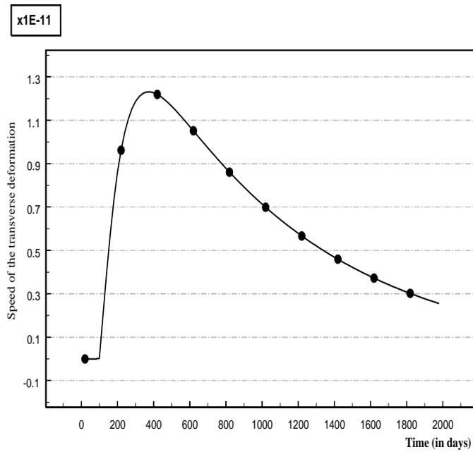
**Figure 3:** Time dependence on the speed of the transverse deformation-Carbon resin epoxy Hercules 3501-5,  $x/thickness=0.5$ ,  $\Delta H = 50\%$ .
