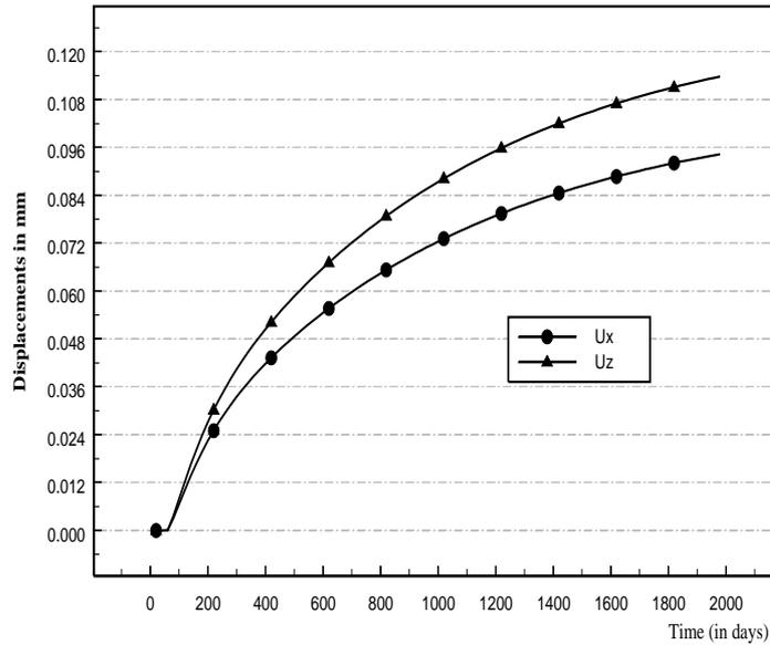
**Figure 6:** Time dependence on the  $U_x$  and  $U_z$  displacements Carbon/Epoxy Hercule 3501-5,  $x/\text{thickness}=0.5$   $\Delta H = 50\%$ .
