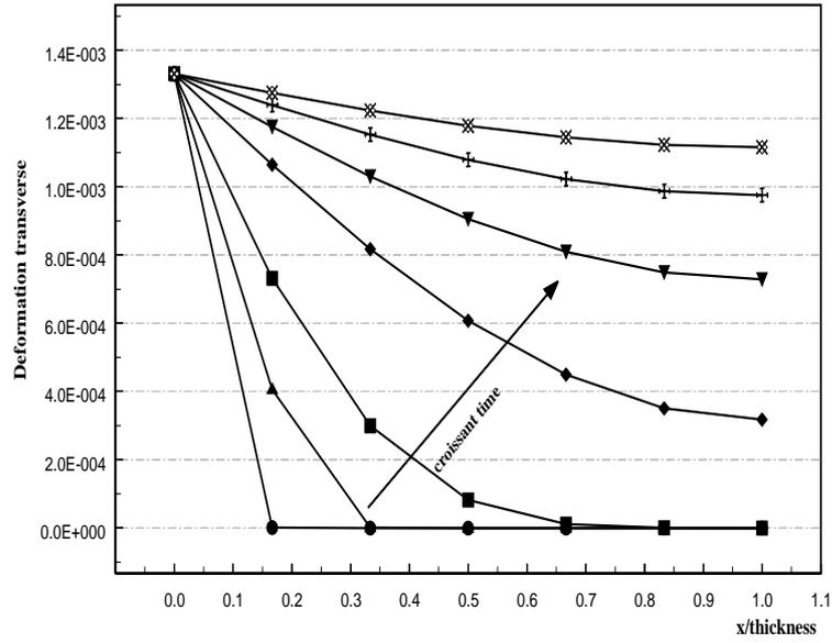
**Figure 4:** Dependence on the thickness on the hygroelastic deformation, Carbon-Epoxy Hercules 3501-5,  $\Delta H = 50\%$ .
