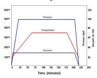
A typical cure cycle for CE3 prepregs is as follows:
