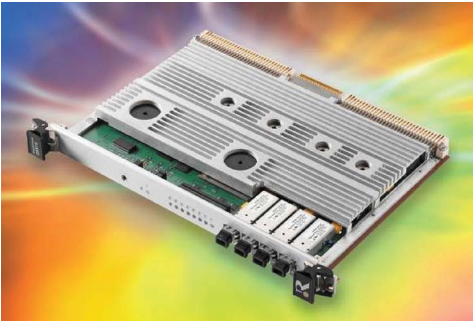
Exhibit 1.5 VME format graphics card showing aluminium heat sink and thermal plugs contacting the top of high-power devices via a flexible interface material (courtesy Radstone Embedded Computing, part of GE Fanuc Embedded Systems)
