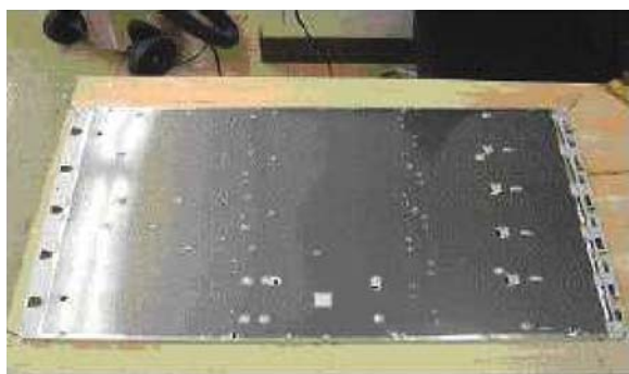
Exhibit 3.6 Spreader retrofitted in Samsung LCD TV (courtesy GrafTech International Ltd)
