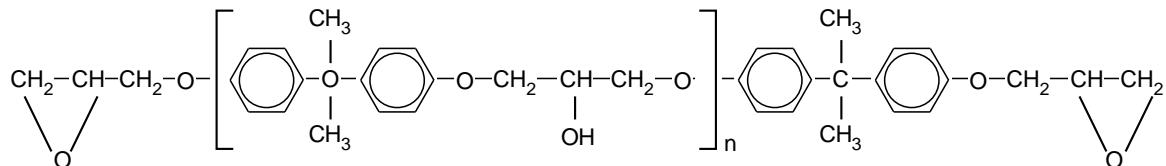
**CY 205** (CIBA - GEIGY) Liquid, unmodified epoxy resin based on Bisphenol A
