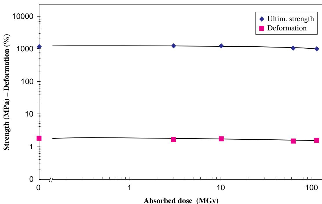
Material: **Carbon-fibre-reinforced epoxy** TIS No. **R 556**
