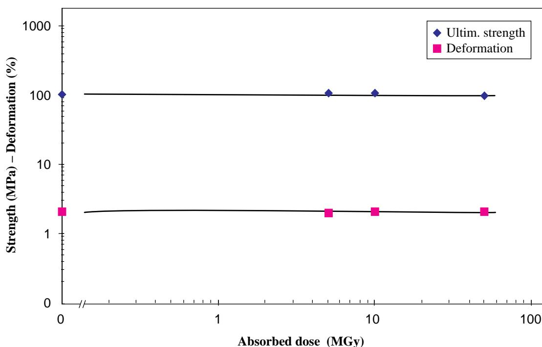
Material: **Polyphenyl oxide (PPO) based plastic** TIS No. **R 491**
