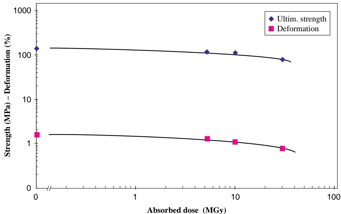
Material: **Epoxy resin (based on Bisphenol A)
