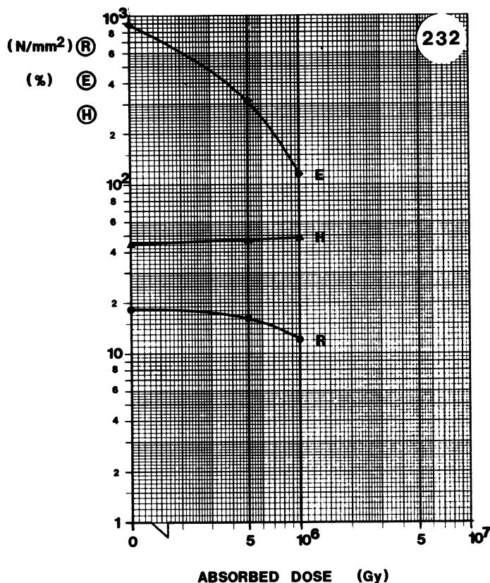
**MATERIAL:** PE**TYPE:** SILYTHENE, HIGH-TENSION, INSULATOR**SUPPLIER:** SILEC**Remarks:** USED FOR SPS 300 kV D.C. CABLE
