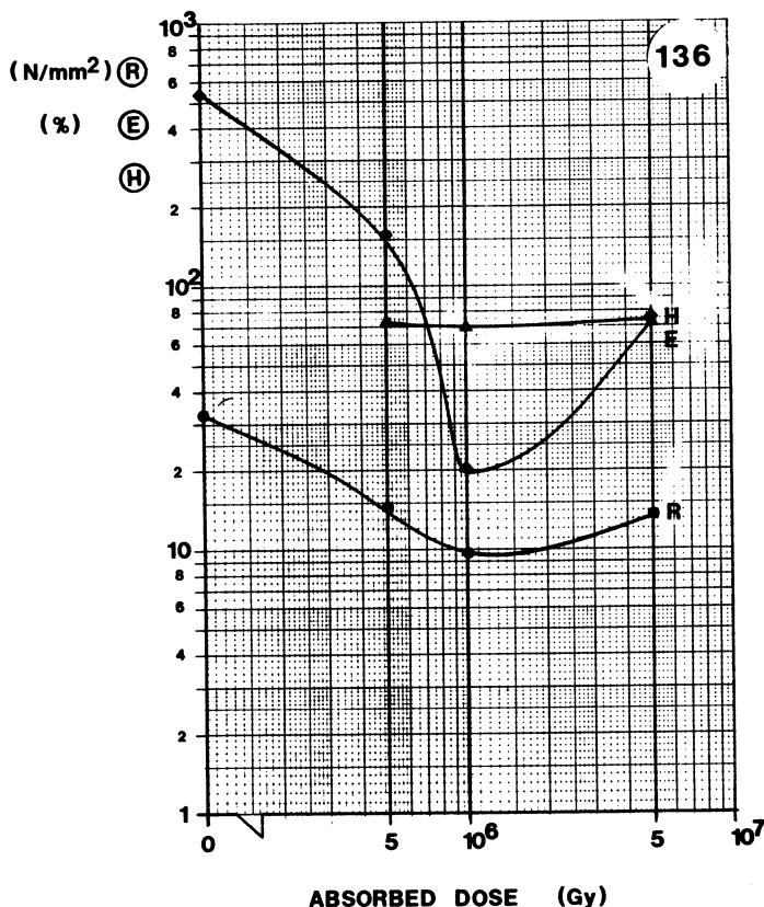
**MATERIAL:** PUR**TYPE:** PUR 3, THERMOPLASTIC**SUPPLIER:** DRAKA**Remarks:**
