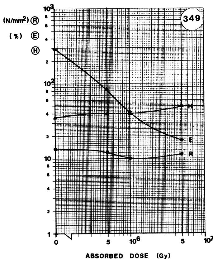
**MATERIAL:** RADOX**TYPE:** RADOX 130**SUPPLIER:** HUBER & SUHNER**Remarks:** FOR SERVICE TEMPERATURES UP TO 130°C
