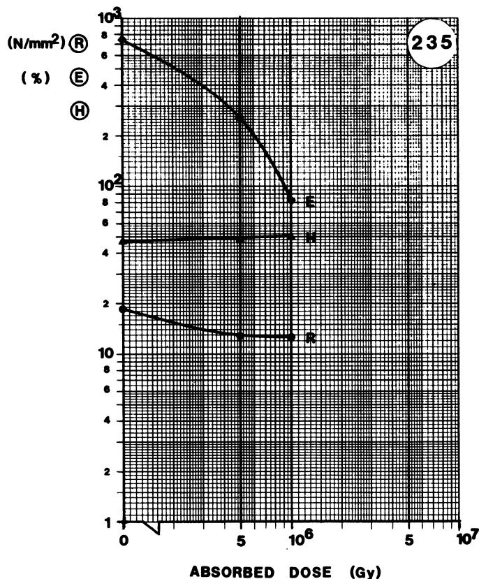
**MATERIAL:** PE**TYPE:** INSULATOR**SUPPLIER:** CABLES DE LYON**Remarks:**
