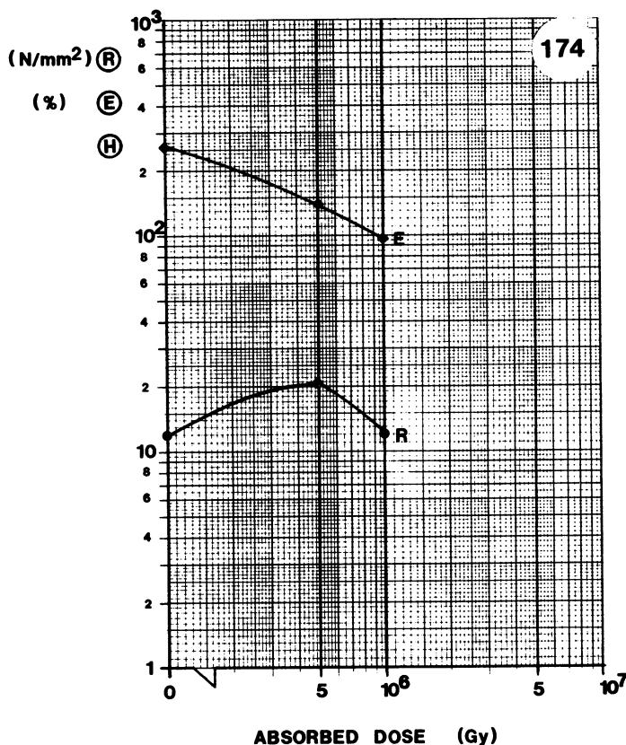
**MATERIAL:** PE**TYPE:** PE/314/PVC**SUPPLIER:** BICC**Remarks:**
