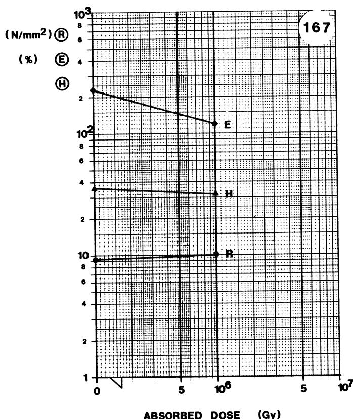
**MATERIAL:** PVC**TYPE:****SUPPLIER:** KABEL-METALL**Remarks:** USED FOR SPS WATER-COOLED POWER CABLES
