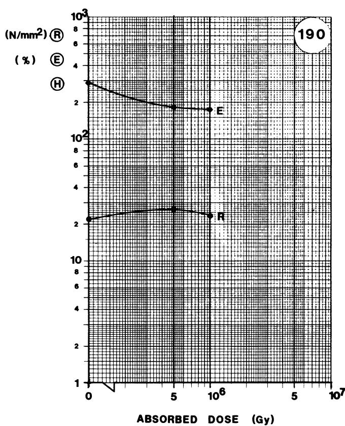
**MATERIAL:** PVC<sub>F</sub>**TYPE:** ANTIRAD**SUPPLIER:** THOMSON-BRANDT**Remarks:** MULTICOR CABLES ND26, ND48, NE10, NE18, NE26, NE48, NF12.
