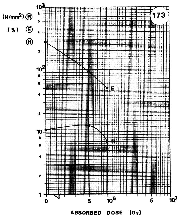
**MATERIAL:** PE**TYPE:** PE/313/PVC**SUPPLIER:** BICC**Remarks:** SPS VIDEO CABLE VA 4 (INDOOR TYPE)
