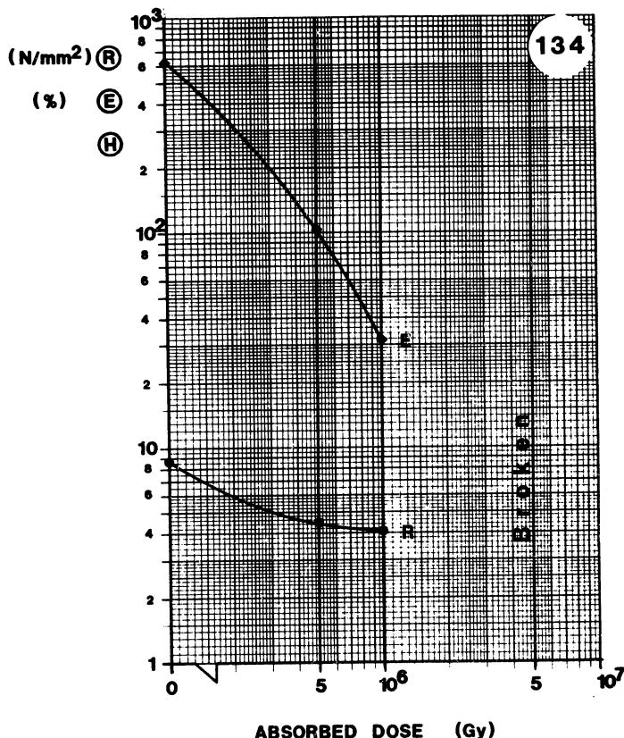
**MATERIAL:** SILICONE RUBBER**TYPE:****SUPPLIER:** DRAKA**Remarks:**
