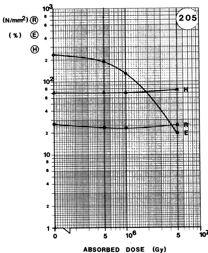
**MATERIAL:** PVC**TYPE:** INSULATOR AND JACKET**SUPPLIER:** FELTEN & G.**Remarks:**
