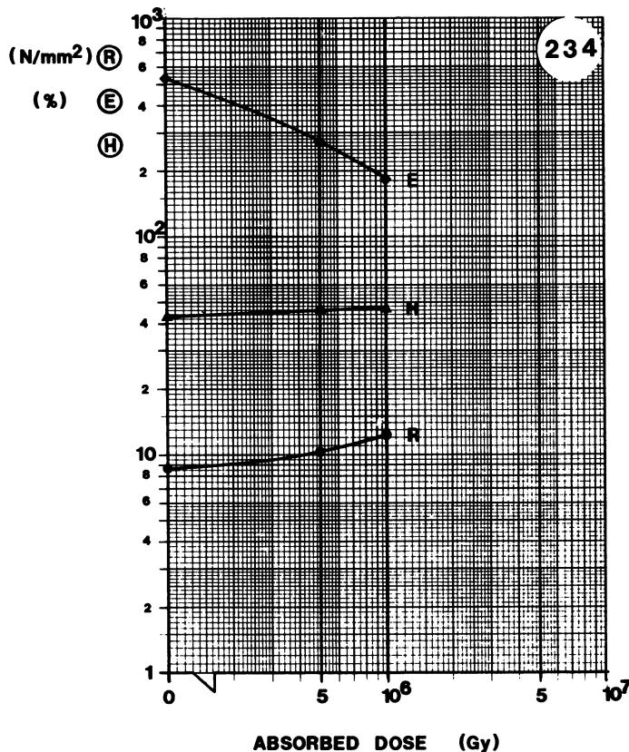
**MATERIAL:** PE**TYPE:** SILYTHENE, HIGH-TENSION**SUPPLIER:** SILEC**Remarks:** CONDUCTING MIXTURE
