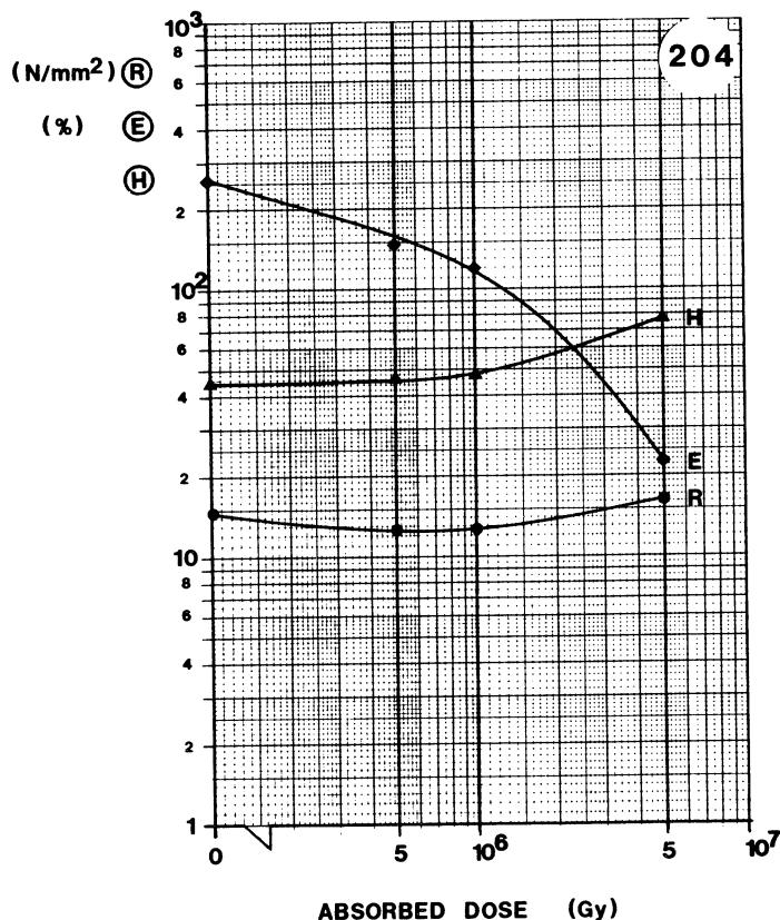
**MATERIAL:** PVC**TYPE:** WITHOUT FILLER**SUPPLIER:** FELTEN & G.**Remarks:**
