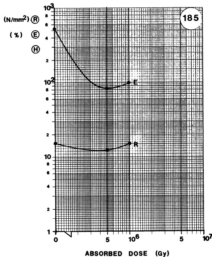
**MATERIAL:** PE**TYPE:** TRANSPARENT**SUPPLIER:** NORSK KF**Remarks:** VACUUM PUMP SUPPLY CABLE SVH2
