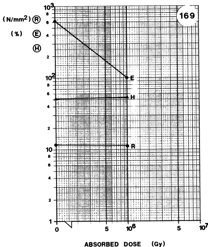
**MATERIAL:** PE**TYPE:** LUPOLEN, JACKET**SUPPLIER:** KABEL-METALL**Remarks:** FLAME RETARDANT; USED FOR SPS WATER-COOLED POWER CABLES
