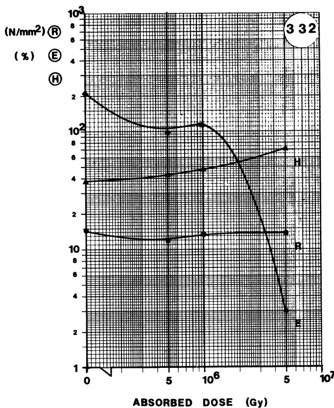
**MATERIAL:** PVC<sub>F</sub>**TYPE:****SUPPLIER:** KABEL-METALL**Remarks:**
