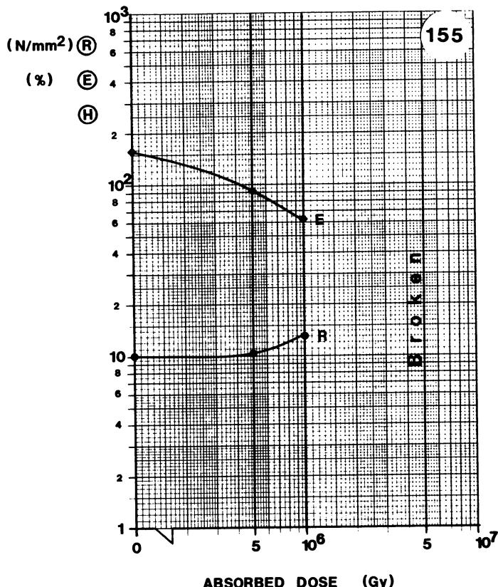
**MATERIAL:** PVC**TYPE:** CHLOROSTOP**SUPPLIER:** KABEL-METALL**Remarks:**
