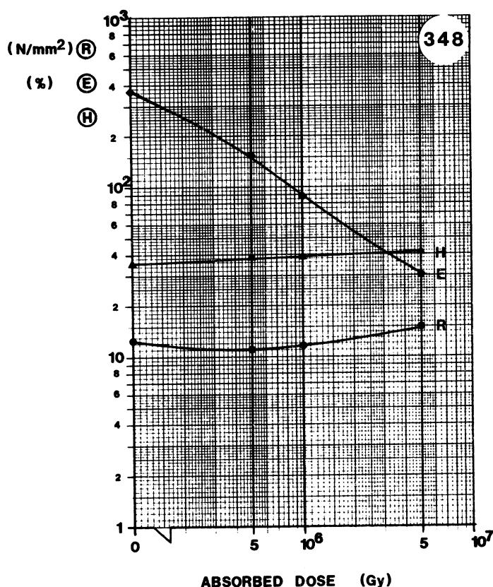
**MATERIAL:** RADOX**TYPE:** RADOX 110**SUPPLIER:** HUBER & SUHNER**Remarks:** FOR SERVICE TEMPERATURES UP TO 110°C
