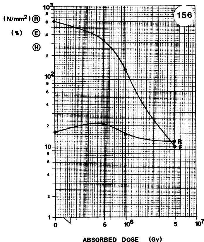
**MATERIAL:** PE**TYPE:** LUPOLEN**SUPPLIER:** KABEL-METALL**Remarks:**
