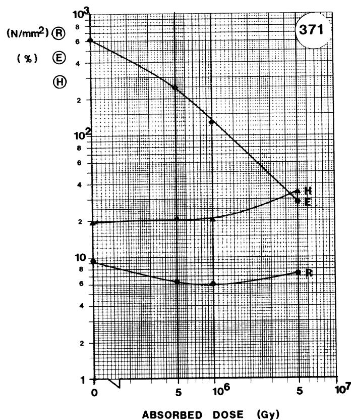
**MATERIAL:** EPR**TYPE:** INSULATOR**SUPPLIER:** KABEL-METALL**Remarks:**
