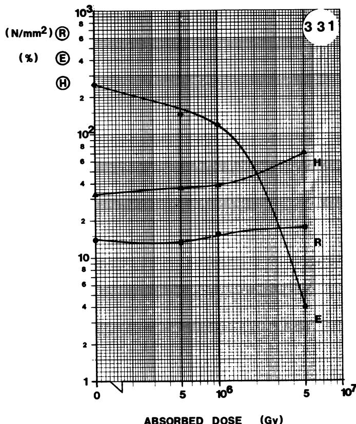
**MATERIAL:** PVC<sub>F</sub>**TYPE:****SUPPLIER:** KABEL-METALL**Remarks:**
