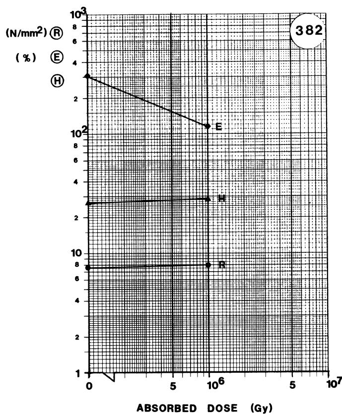
**MATERIAL:** EPR**TYPE:** JACKET**SUPPLIER:** ALFACAVI**Remarks:** USED FOR 1 kV, 400 MM<sup>2</sup> AL CABLES, SPS
