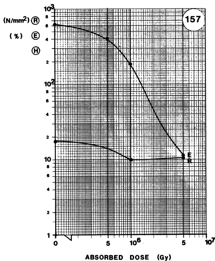
**MATERIAL:** PE**TYPE:** STABILIZED**SUPPLIER:** KABEL-METALL**Remarks:**
