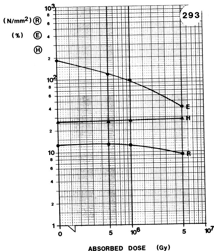
**MATERIAL:** EPDM**TYPE:** INSULATOR**SUPPLIER:** DÄTWYLER**Remarks:**
