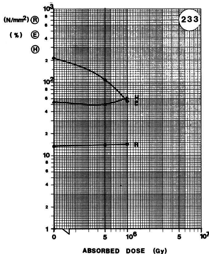
**MATERIAL:** PE**TYPE:** SILYTHENE, HIGH-TENSION**SUPPLIER:** SILEC**Remarks:** CONDUCTING MIXTURE EXTRUDED ON
