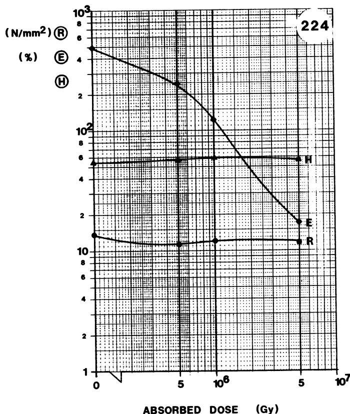
**MATERIAL:** PE**TYPE:** INSULATOR**SUPPLIER:** HUBER & SUHNER**Remarks:**
