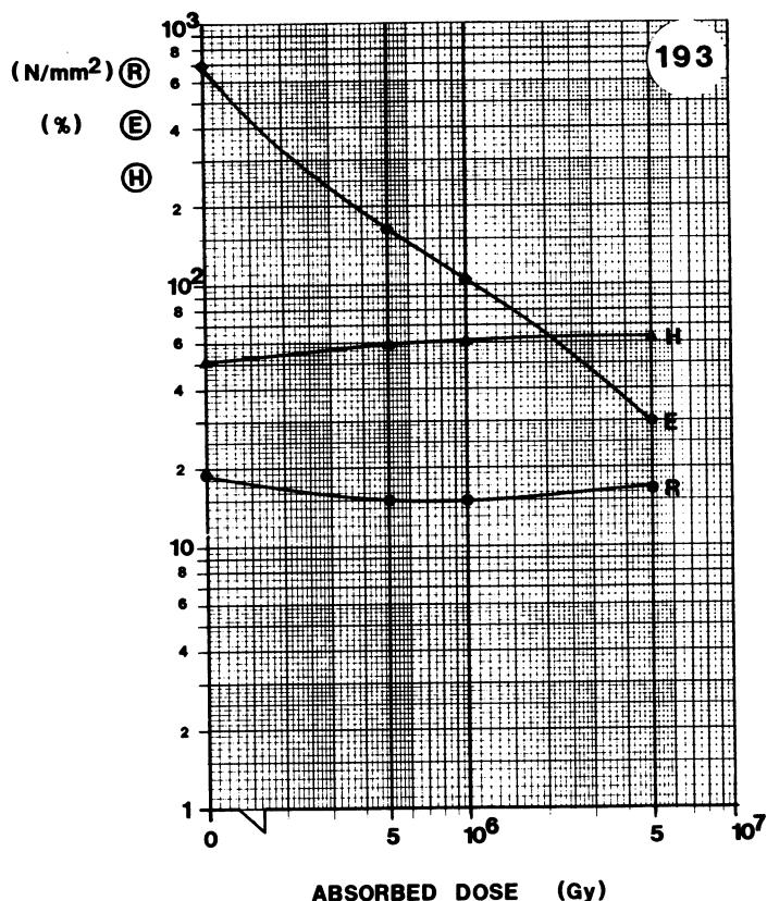
**MATERIAL:** PE**TYPE:****SUPPLIER:** SIEMENS**Remarks:**
