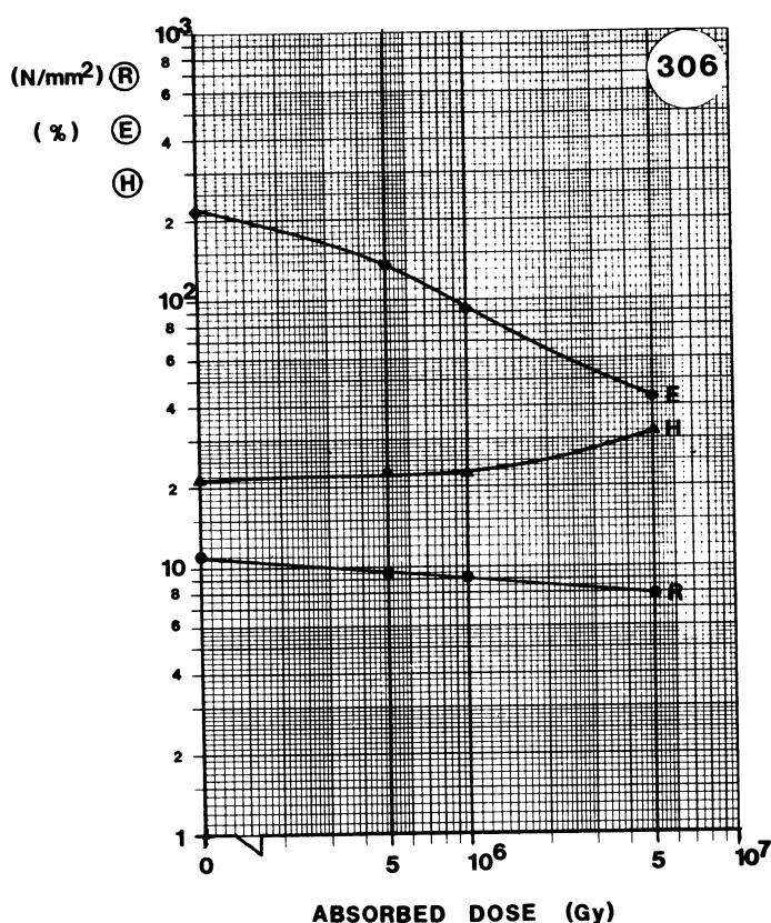
**MATERIAL:** EPDM**TYPE:** NORDEL, FLAME RETARDANT**SUPPLIER:** DOLDER**Remarks:**
