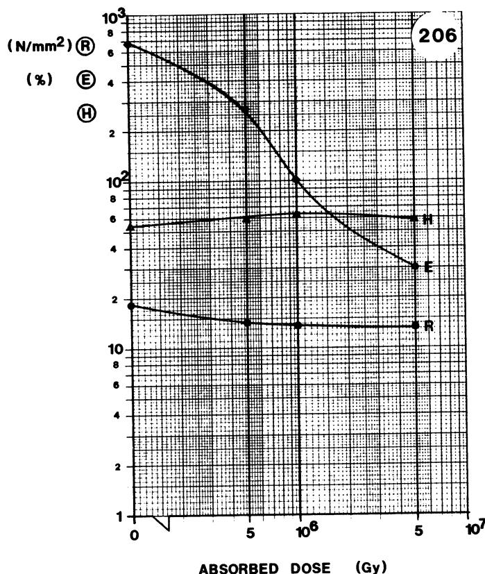
**MATERIAL:** PE**TYPE:** LUPOLEN**SUPPLIER:** FELTEN & G.**Remarks:**
