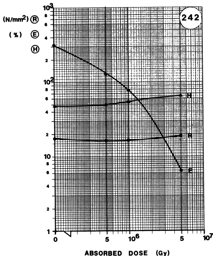
**MATERIAL:** PVC<sub>F</sub>**TYPE:** JACKET**SUPPLIER:** THOMSON-BRANDT**Remarks:** USED FOR SPS 1 kV POWER CABLES
