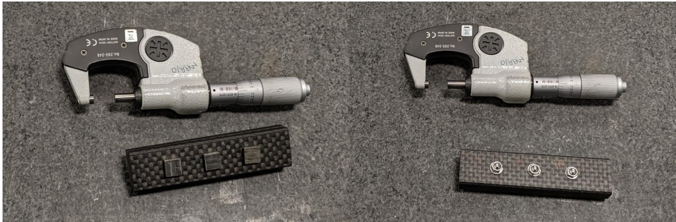
Figure 48 Specimen for preload loss measurement. A total of 6 bolts were bolted in this configuration.
