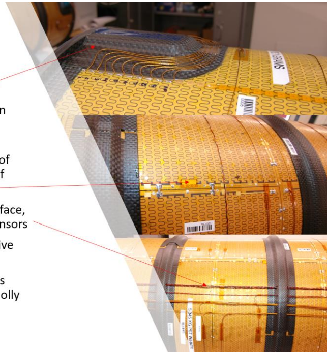
Figure 6 External Connectivity of Heaters and Ground Plane
