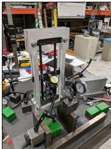
Figure 42 Radial loading configuration and measured displacement
