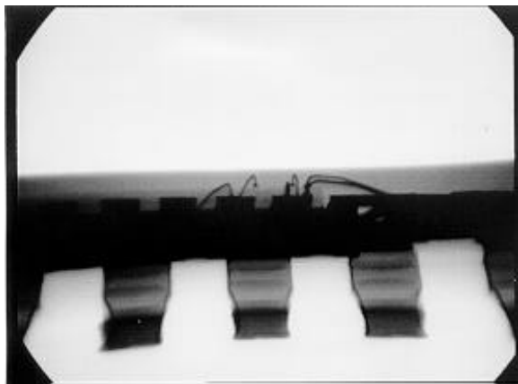
Figure 2. Samsung 32MB Flash Static Random Access Memory (SRAM). Note the close proximity of the bond-wire loop to the top surface of PEM.
