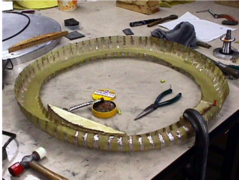
Figure 1. The brass screen during fabrication.
