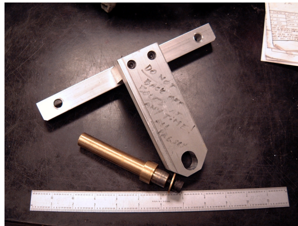
Figure 6. One of the alignment fixtures for the glue-up procedure.
