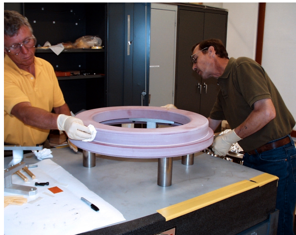
Figure 8. Final alcohol wipedown of the epoxy casting (Left) and slip flange surfaces (Right).
