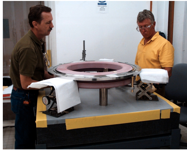
Figure 9. Using lab jacks to raise and lower the slip flange onto the casting (both left and right).
