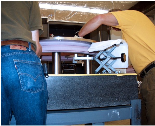
Figure 9. Using lab jacks to raise and lower the slip flange onto the casting (both left and right).
