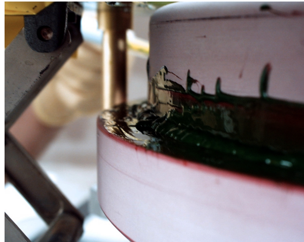
Figure 10. Application of the Hysol® adhesive (left), and a detail of the spread-out adhesive (right).
