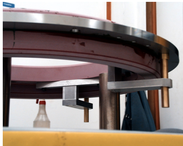
Figure 11. The flange, lowered onto casting (left), and a view from below (right). Note the fixtures.
