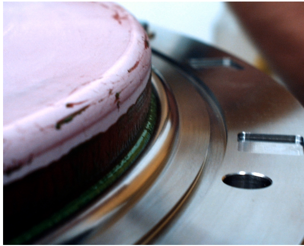
Figure 12. After lowering the flange, the air pockets and excess epoxy were squeezed out (left). This excess epoxy was wiped and scraped away (right), especially in the triple-point radius shown at left.
