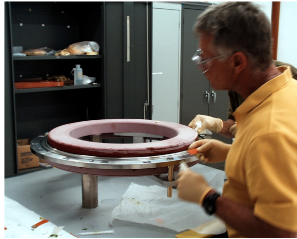
Figure 12. After lowering the flange, the air pockets and excess epoxy were squeezed out (left). This excess epoxy was wiped and scraped away (right), especially in the triple-point radius shown at left.
