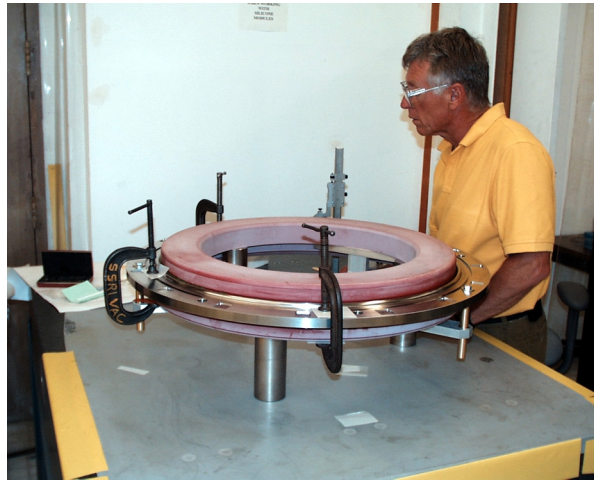
Figure 13. A height gauge and C-clamps were used to level the flange with respect to the casting. The assembly was allowed to fully cure before the clamps were removed.
