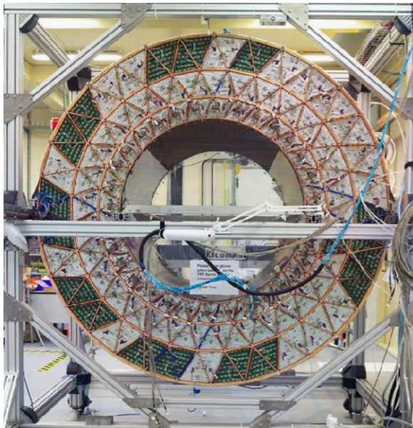
Fig. 16. TRT barrel during final attachment of cooling and electrical services (from [66]).
