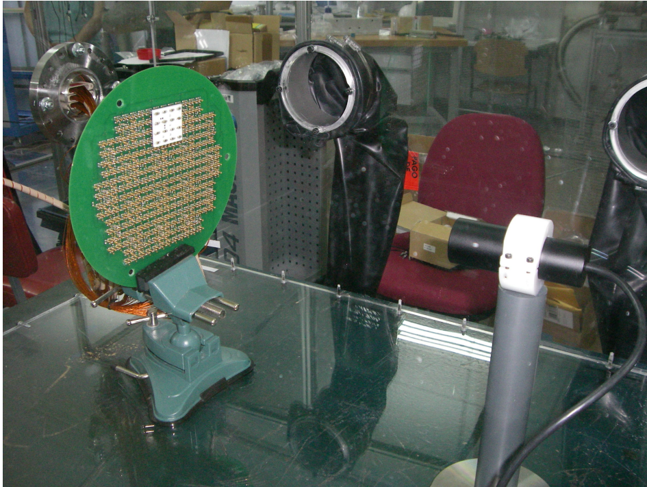
Figure 4.15: The SiPM plane inside a test box, made of acrylic.
