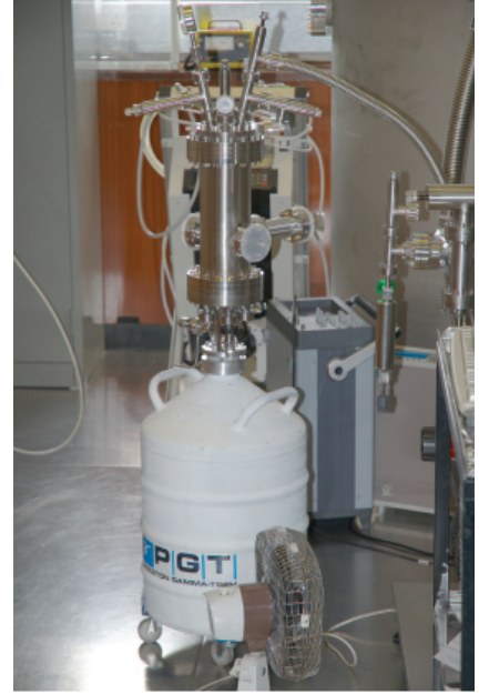
Figure 8.16: Photograph of the ZEPLIN III electron lifetime monitor positioned on the liquid nitrogen cryostat.
