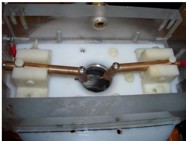
Figure 3.2: Lexan gas chamber and electrodes for surface flashover studies.
