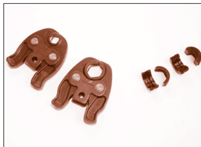
FIGURE 58: Pressing jaw selections
