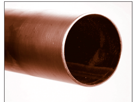
FIGURE 36: Clean and smooth tube end
