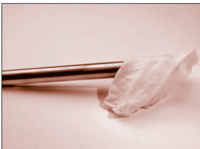
FIGURE 84: Wipe with premoistened alcohol wipe or pad
