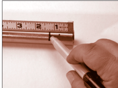
FIGURE 85: Marking insertion depth
