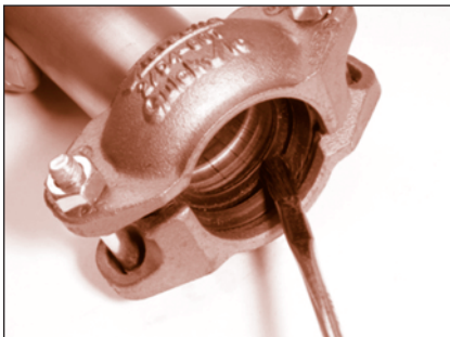
FIGURE 40: Applying lubrication to gasket
