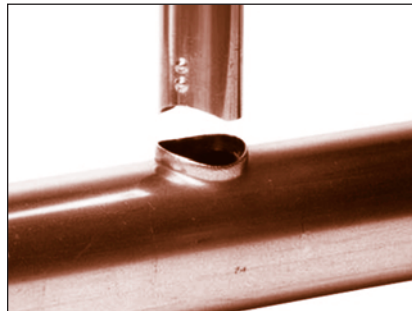
FIGURE 103: Aligning the dimples with the run of the tube
