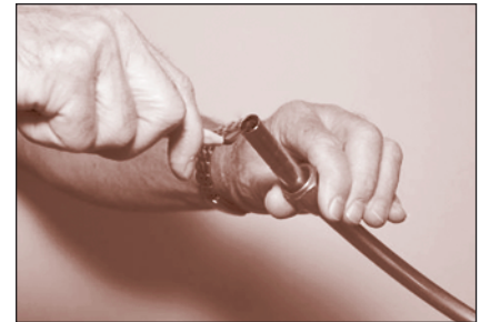
FIGURE 30: Reaming prior to flaring the tube end
