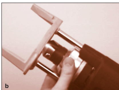
FIGURE 95 (a and b): Retracting the forming pins
