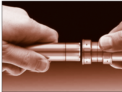
FIGURE 72: Aligning tube end squarely
