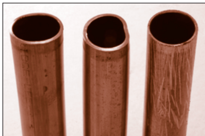
FIGURE 45: Inspect tube for imperfections
