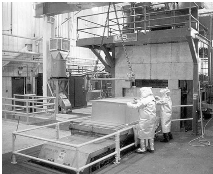
Fig. 9 Loading a sheet of titanium into a superplastic forming die
