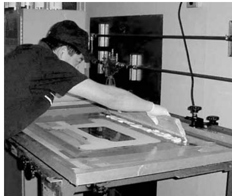
Fig. 11 Typical silk screen application of the stop-off material
