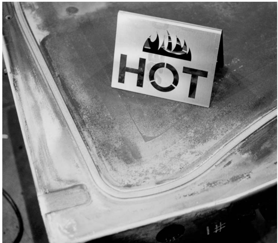
Fig. 5 Typical tool finish after being exposed to elevated temperatures. This hot forming die has a heavy scale and oxide layer caused by long exposure to high temperatures. Dies must be cleaned using abrasives in between production runs in order to avoid mark-off being transferred to the part surface. The light area is alpha case that has been migrated to the die from the titanium parts.
