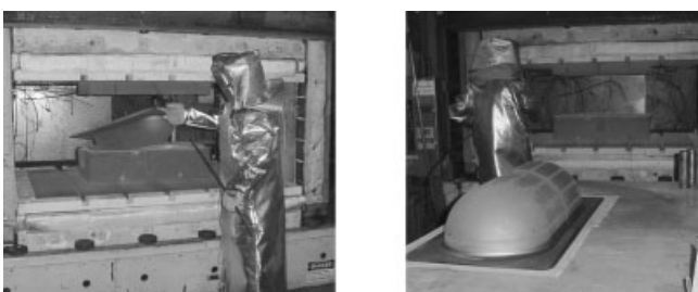
Figure 7. The SPF fabrication of zepelin pan test parts is shown. Left: An operator removes a hot part out of the zepelin die. Right: A finished zepelin pan that has cooled is shown on a table in front of the hot die.
