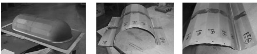
Figure 7. The SPF fabrication of zepelin pan test parts is shown. Left: An operator removes a hot part out of the zepelin die. Right: A finished zepelin pan that has cooled is shown on a table in front of the hot die.
