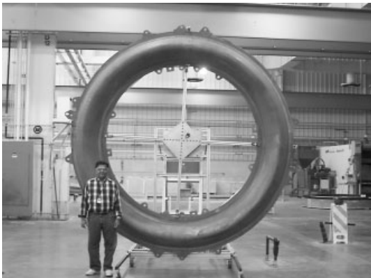
Figure 10. A successfully formed approx. 4 meter diameter titanium engine inlet Lipskin test part.
