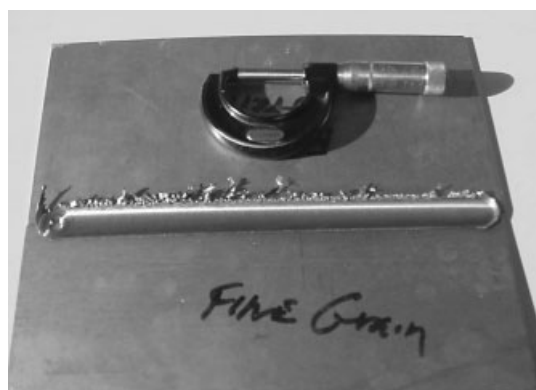
Figure 4. Titanium FSW produces a much larger burr than aluminum FSW, which is about 0.2 mm thick and very sharp. Note that the start of the weld is completely encased with titanium, while a hole is left behind at the end of the weld because of the extraction of the rotating pin.
